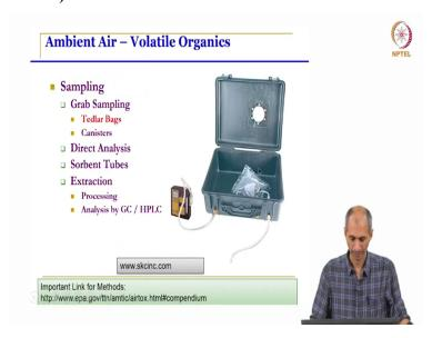
So here, this is the other one, this is the Tedlar bag that I was talking about. There's a bag and this is kept inside a vacuum and then sampling is done into the bag using a pump.
