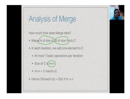
So, in each iteration notice that we add one element to C, but the size of C is exactly m plus n, because there are m elements in A and there are n elements in B and each of them will eventually make it to C. So, there are m plus n elements and in each iteration of this loop, the loop that we had before, in each iteration of this loop, one element gets added to C, either in this if or in this if, k is incremented.
