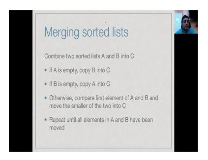
So, in order to analyze merge sort, we first need to look at the merge operation itself. So, remember that when we merge two sorted list, what we do is, we take both list side by side and we keep copying the smaller of the two elements at the header each list into the final list C.
