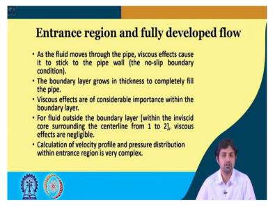
Now, as the fluid moves through the pipe, viscous effects cause it to stick to the pipe wall because of the no slip boundary condition. As I told you here, as it starts moving because of the no-slip boundary condition, the viscous effect will cause it to stick to the pipe wall and the boundary layer will grow in thickness to completely fill the pipe. Now, the viscous effects are of considerable importance within this boundary layer, as we had discussed.
