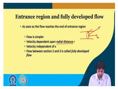
So, as soon as the flow reaches the end of the entrance region, the flow becomes simple, much more simple and the velocity will be dependent upon the radial distance r and the velocity will also be independent of x. What is r? So, this is a pipe., so this is x and because it is a pipe, it is circular, so this is r, radial distance from the center line. The flow between section 2 and 3 is called fully developed flow.
