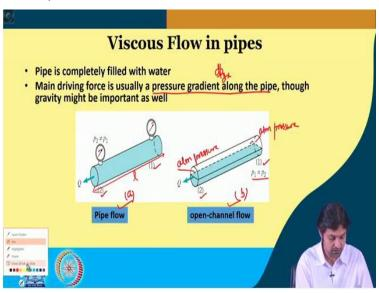
So, to get started, one of the important things that you must know that the flow in the pipes are viscous in nature. Therefore, we call it viscous flow in pipes. So, an important property of a pipe flow is that the pipe is completely filled with water or any other fluid, whichever it can be; it can be with oil or anything, but the pipe should be completely filled with it. Here, the main driving force is usually a pressure gradient along the pipe.
