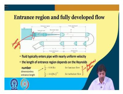
Now, there is an entrance region and fully developed flow. We should talk about this what entrance region is and what a fully developed flow in a pipe flow is. So, you see, there is a figure here, which I will explain it to you later. So, there is a pipe coming out from the reservoir and the, so this is the and this is pipe. So, as soon as the water comes out from the reservoir to the pipe, earlier there was no water.
