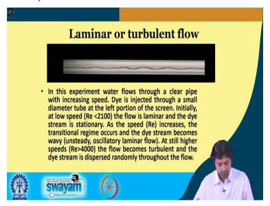
So, this is a figure of an experiment. The link I have written, I have not attached the video because of the copyright issues. But this is an image of the experiment, which was done in the pipe, as I have shown you. And this has been done with the help of a dye. So, what happens is, in this experiment, the water flows through a clear pipe. So, there was a clear pipe and the speed has been increased in steps.
