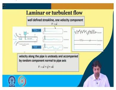
So, now, when the flow in the pipes occur, the important question is, whether it is laminar or turbulent flow because that is one of the classification of the flows that we also saw in the open-
