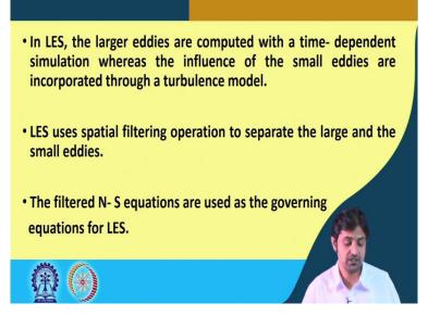
So our domain size does not is not mean we do not need to be, you know, accounting for the smaller eddies. We make our grid size that it captures the largest of the eddies. So, LES uses spatial filtering operation to separate the large and the small eddies as I have told you and the filtered navier stokes equation are used as the governing equation for large Eddy simulation.
