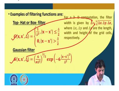
So examples of filtering functions are there is a top hat or box filter, where g x see, you see there is a G here, this is a filtering function and this therefore this is a filtered function. So g xx can be given by different box filter, it is a different study in its own is a Gaussian filter. So remembering the name of the filter is good enough you do not need to remember those equations. So for 3d computation, the filter with this is important.
