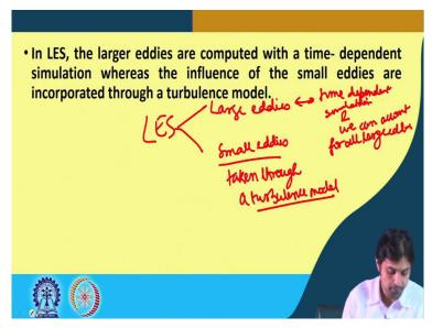
So, in LES the larger eddies are computed with a time dependent simulation where the influence of this small eddies are incorporated through turbulence model. So, we say in LES 2 parts large Eddies and there are small eddies. So they are solved through time dependent simulation and we account for everything for all large eddies but small eddies are so much the, the effects of the small eddies is taken through a turbulence model.
