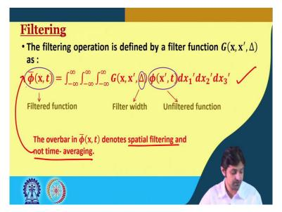
Now the filtering the filtering operation that we have talked about is defined by a filter function g of x, x dash, delta as it is a very complex but there is a filtering operation that you must know that in LES we use a filtering operation to cut off the smaller eddies and solve in reality for the larger eddies and then approximate this smaller eddies is using the turbulent model. So this is a filtered function delta is a filter with which is mostly said to the size of the mesh.
