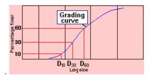
To obtain the grading characteristics, three points are located first on the grading curve.
