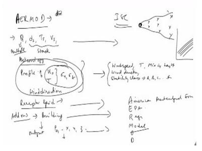
The big difference between ISC and AEROMOD, the ISC is the older version. They are both similar. So here again, you need same kind of information, the information that you need is the Q the rate, you need the diameter of the source, you need temperature of the source, you need velocity of the source, these are all stack; stack diameter, stack temperature, stack velocity. Then you need meteorological conditions.
