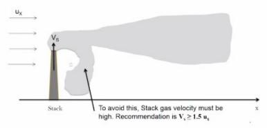
Due to low pressure just downwind of the stack, there might be suction from the plume causing exposure to the receptors there
