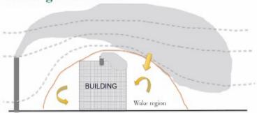
The presence of a BUILDING in the path of air causes streamline separation resulting in the formation of low pressure regions called "wakes". These can pull in the pollutant plume from a different source. Alternatively, sources on top of the building that are within the wake will circulate locally causing higher concentration and exposure.
