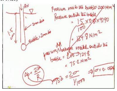
So, what it says is so, this is water and this is air is coming here. This is the bubble that is 2 mm diameter. This is 2 mm diameter and this is 1.5 cm. Okay. So, the pressure inside the bubble is
