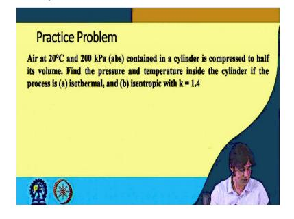
Now we go to our next problem that is related to the air and the compression so, mostly related on the gas laws. So, air at  $20^{\circ}$  and  $200 \ kPa$  contained in a cylinder is compressed to half its volume. Find the pressure and the temperature inside the cylinder of the process (a) isothermal and (b) if it is isentropic with k = 1.4. So, okay, the best way to go is to have the whiteboard. So, whiteboard is very good.
