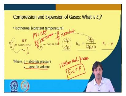
So, compression and expansion of gases. So, one of the phenomenon's is isothermal, which is constant temperature. So, what happens is PV = nRT, that equation we already know So,
