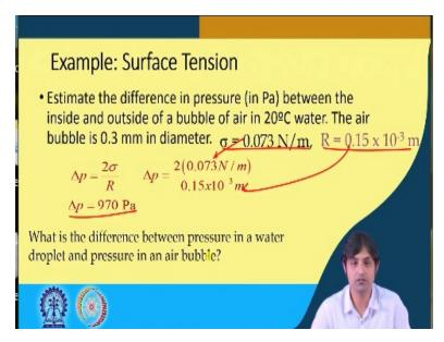
So, we have included an example of surface tension here, but, estimate the difference in pressure between the inside and outside of bubble of air in  $20^{\circ}$  water  $20^{\circ}$  of water. The air bubble is 0.3 *mm* in diameter. So, we already know the equation here  $\sigma$  is given as 0.073 N/m and R is the radius 0.15 \*  $10^{-3}$ .
