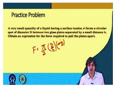
So writing the final equation here F. F that is required will be  $F = \frac{\pi D}{2\hbar} \sigma D$ ,
