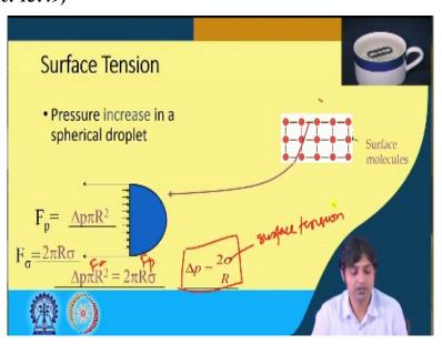
Another such properties, the surface tension. An example here is that the pressure increases in a spherical droplet, this is the surface of a droplet for example, and this is yeah, surface molecules
