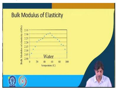
So, this is the figure, which shows the bulk modulus elasticity how it varies with the temperature. So, as you can see the bulk modulus elasticity increases as the temperature increases to a certain value and then starts to decreasing these are the normal ranges of temperature in air, 100 degrees is very rare but the most common ones are 0 to 30 degrees in India it can be 0 to 40 degrees. So, for water, so, I am sorry this bulk modulus elasticity is for water.
