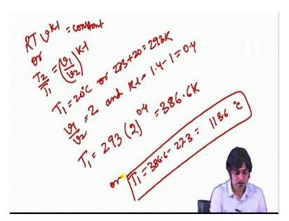
So if we use so what we found out in the last screen was RT v to the power k - 1 is equal to constant or we are also able to write  $T_2 / T_1$  because R will be canceled on both sides,  $(V_1 / V_2)^{k-1}$ . We know that  $T_1$  was  $20^{\circ}$  or in Kelvin, it is going to be 273 + 20 is equal to 293 K and  $(V_1 / V_2) = 2$ . And k - 1 will give out 1.4 - 1 as 0.4.
