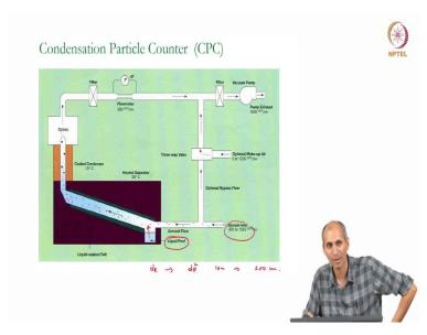
So, that method of measurement called as a condensation particle counter (CPC). These small nanoparticles you don't have a way of counting it yet. So, but you will know how to count particles that are in the range of sub about 0.3 microns 0.4 microns. So, this is using the scattering instrument, which we already saw that the limited there is about 0.3, 0.2 microns. So, you allow the nanoparticle to grow to that size.
