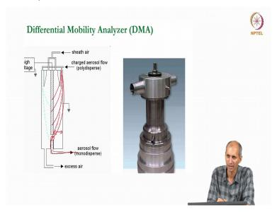
So electrical mobility, and the instrument that is used to make is called as a differential mobility analyzer. And this instrument, what it does is it charges all the particles coming in. But
