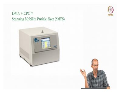
So, very complicated instrument, the entire thing is called as a scanning mobility particle sizer or SMPS very expensive instrument cost around 50 lakhs, 60 lakhs as you can imagine, but it is used a lot in trying to understand what is the distribution of particles all the way from 10 nanometers up to 10 microns, you can do the entire thing in 1 sweep.
