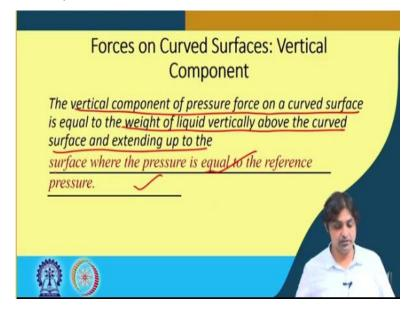
So, to sum the vertical component of the pressure force on a curved surface is equal to the weight of the liquid vertically above the curved surface and extending up to the surface where the pressure is equal to the reference pressure. This is the thumb rule. So, the vertical component of the pressure force on a curved surface is equal to the weight of the liquid vertically above the curved surface, okay. And extending up to the surface where pressure is equal to the reference surface.
