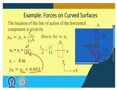
The location of the line of action of the horizontal component is given by  $y_R = y_c + \frac{I_{xc}}{y_c A}$ . This is what we have seen before here, h c is equal to y c, the height of the centroid is the actually also the y because we have assumed an axis in the vertical direction. So, y R is going to be y c + if you look at this, so,  $\frac{I_{xc}}{y_c A}$  will come out to be, you know, because of a square / 12.
