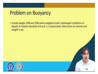
The problem says, the body weighs 20 Newton and 10 Newton when weighed under submerged conditions in the liquid of relative densities 0.8 and 1.2 respectively. Determine its volume and weight in the air. So, yeah, what I am going to do again a screen it is very simple problem, but I think it will give you a thorough brush up. Let, I have not selected the pen. Now, I will select the screen, white screen.
