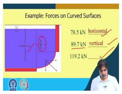
So, now to sum up, this is the horizontal force 78.5, this is 89.7 the vertical force and 119.2 is the resultant force and, yeah. The distances are shown, .948 meter that we have calculated you know 4.083 meter also we had calculated. So, this solves our this problem of forces on curved surface. So, this will, you know, give an overall picture of what is happening in this, you know, forces on curved surface.
