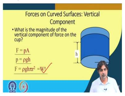
So, this is one of the examples. My question to you is what is the magnitude of the vertical component of force on the cup? Tell me? Force is pA, correct. Pressure is  $\rho gh$ , putting it  $\rho gh$ , area is  $\pi r^2$ , and this actually is the weight of the liquid supporting it. So that will be the force, vertical force.
