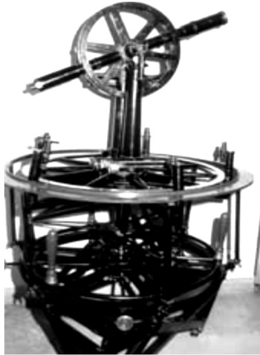
Figure 1.3 The 36 inch theodolite used in the Indian triangulation (Keay, 1983)
