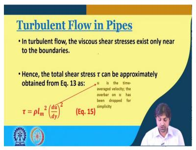
So, now we will see the turbulent flowing pipes now. So, in turbulent flow the viscous shear stresses exists only near the boundary and most of the region is dominated by the turbulence. So, near the boundary the viscous shear stress will act and that are the only places where its existence is. Hence, the total shear stress can be approximately obtained from equation 13 as the total, you know, this was so, this was equation 13.
