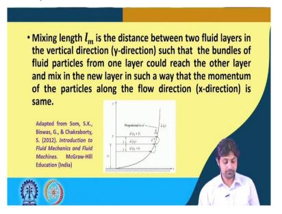
So, mixing length 1m, he said it can be described in terms of mixing length 1 m. He said mixing length 1 m is the distance between 2 fluid layers in the vertical direction, in the y direction, such
