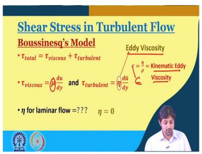
So, we are going to continue with this particular topic. So, shear stress in turbulent flow. We are going to talk about a model that is called Boussinesq's model, where the total shear stress, in case of laminar flow it was due to the viscosity viscous. Sorry. Yeah, that was only due to the viscous. But in a turbulent flow, there is an additional component of shear stress that happens because of the turbulence in the flow.
