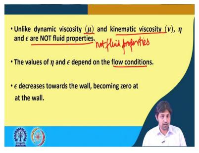
So, unlike the dynamic viscosity mu and kinematic viscosity nu, eta and epsilon are not fluid properties, they are not fluid properties. The values of eta and epsilon are dependent on the flow conditions. So, epsilon decreases towards the wall becoming 0 at the wall. So, the epsilon, that is,
