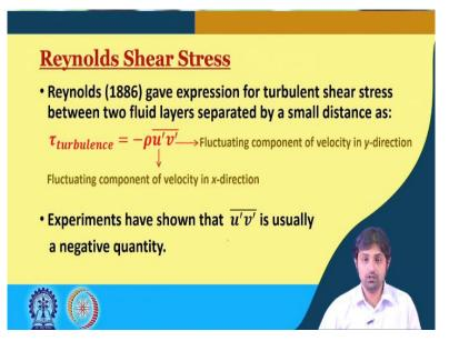
Now, coming to what is Reynolds shear stress. So, Reynolds in 1886 gave expressions for turbulent shear stress between two fluid layers separated by a small distance. And he said that the shear stress due to turbulence can be written as, minus rho u prime v prime whole bar. Actually, it is not an assumption, but this can actually be derived, which we will do at some point in this hydraulic engineering course, but not now.
