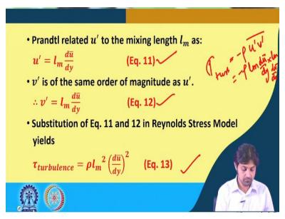
So, Prandtl related u prime to mixing length lm. He said that this u prime, as you can see in the figure here, he said proportional to u prime but I am going to write it in the next slide. He related u prime to the mixing length lm as, he said this u prime can be written as, mixing length lm multiplied by the gradient of the average velocity. So, he said u prime, this is very important to know, lm as the du bar / dy.
