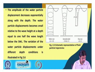
So, you see, this is the representation the schematic representation of fluid particle trajectories the amplitude of the water particle displacement it first of all it decreases exponentially along the water depth the water particle displacement becomes small relative to the wave height at a depth equal to one half the wavelength below this still water level that is the deep water the variation of the water particle that displacement under the depth condition is illustrated in this.
