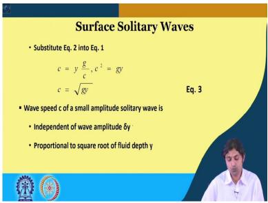
So, if we substitute equation 2 into equation 1, so c is equal to y delta V / delta y, we get c is equal to yg / c and c can go this side it becomes c square is equal to gy, or the final equation c is equal to  $\sqrt{gy}$ . Where c is speed of small amplitude surface solitary waves, g is acceleration due to gravity and y is depth of water in open channel. And this is equation number 3.
