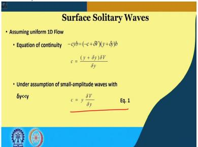
Welcome back students. In the last lecture we left off by deriving this equation 1, for surface solitary waves and we will continue from this point onwards. So, as we saw if when we applied the equation of continuity to that control volume, we arrived at an equation given by c is equal to y delta V / delta y.
