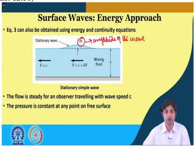
The energy balance approach. So, the equation number 3, c is equal to under root gy can also be obtained using energy and continuity equations instead of momentum. So, you see this simple stationary simple wave. So, when the observer is moving with the wave to him, this is, I mean, it is moving with the same wave speed. So, this wave will appear to be stationary to the observer, other things are same.
