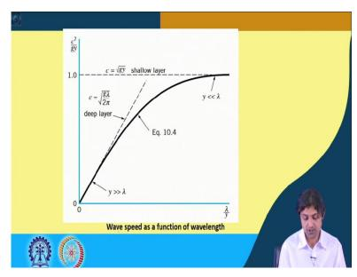
This is a graph that actually shows, you know, the curve that has been plotted lambda / y So, y is the depth and lambda is the wavelength and c is the speed of the wave, y is the depth and you see, this is the curve, different regimes have been shown. So, this is deep water. So, deep water when somebody says it is assumed that the depth of the water is much, much larger than the wavelength, shallow water means that the depth of water, depth and this is wave length.
