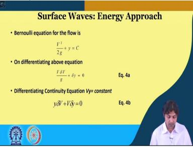
Now, we apply the Bernoulli's equation for the flow. Bernoulli's equation says that because there is the pressure is constant, so the pressure term will vanish, so it will become  $\frac{V^2}{2g} + y$  is equal to constant. This is Bernoulli's equation So, if we differentiate this above equation, so what we get when we differentiate this with respect to y, so we get V square will become, so I will try to define 2V delta V and 2g will remain the same.
