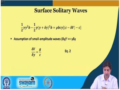
So, the we apply the change in momentum, we change, rate of change of momentum is the force. So, we obtain half gamma y square b, that is, force on the right hand side minus force on the left hand side is equal to rho b c y mass flow rate. You remember from momentum equation of fluid dynamics and this was obtained from Reynolds transport theorem. So, mass flow rate into the velocity change. So, the left hand side had c - delta v and the left hand side was and this was the right side.
