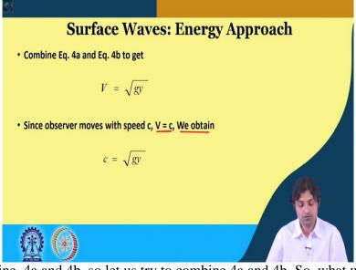
And if we combine, 4a and 4b, so let us try to combine 4a and 4b. So, what we do is, so the 4 a let us see, V / g is equal to - delta y / delta V from 4a. And from 4b, we can write, V delta Y is equal to - Y delta Y. And if we bring this down it is become delta Y delta Y is equal to - Y. And we put this one here. So, we are going to get Y g is equal to minus of minus becomes plus, so this will become Y and this will become Y square is equal to Y.
