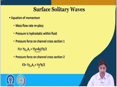
So now, we proceed further, we have applied equation of continuity now, we should also apply equation of momentum. So, how to apply? So, the mass flow rate m is given by ρbcy, ρ
