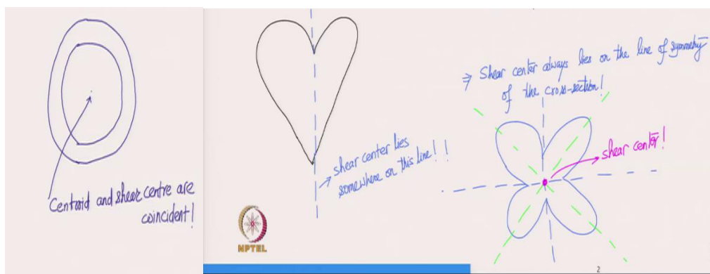
Figure 3: (a) annular cross-section having infinite lines of symmetry (b) heart-shaped cross-section having one line of symmetry (c) Flower shaped cross-section having four lines of symmetry
