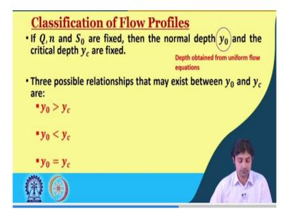
So, now the classification of flow profiles. What are the flow profiles in gradually varied flow? So, if the flow rate Q, Manning's number n and S0 are fixed, then the normal depth y0 and the critical depth yc is also fixed. You understand this? See, Q is equal to 1 by n A, sorry, I will just, sorry, the Manning's equation is V by n S to the power 1/2 Rh to the power 2 by 3 alright.
