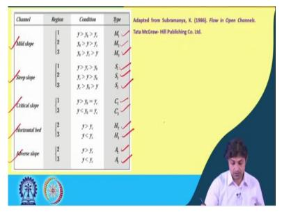
So, there can be 3, you know, as we have already seen that the profiles, there is mild slope, there is steep slope, there is critical slope, there is horizontal bed and the adverse slope. So, depending upon the 3 regions, you know, there could be 3 different types of profiles. If, y is greater than, so region 1 is called M1, region 2 is M2, you know, region 3 is M3, same S1, S2, S3, C1 and C3 and this one is H2 and H3 and this adverse slope is A2 and A3.
