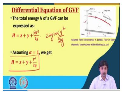
Now, what the going to the differential equation of the gradually varied flow. So, first we have to draw, you know, figure the; I have shown you a figure here, where there is a small bed slope, there is a channel with a small bed slope S 0, so basically, this theta is the angle, the datum is given by this, you know, this is the datum and the height at any in the height of the bed, at any point is at a distance z from the datum.
