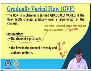
So, to get started, we should understand what exactly a gradually varied flow is. We have already derived an equation before, but to make it more clear we will see it in a little different way, a derivation of a different sort. So, what is gradually varied flow? The flow in a channel is termed as gradually varied, if the flow depth changes gradually over a large length of the channel.
