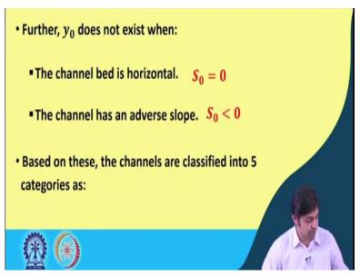
Further, y0 does not exist when, I mean, there will be no y0, if the channel bed is horizontal, that means, S0 is equal to 0. The channel if it has an adverse slope then, also there will not be any normal depth, that means, S0 is less than 0 and based on these, the channels, so based on these, you know, conditions the channels are classified into 5 categories, the channels itself. (**Refer Slide Time: 19:50**)
