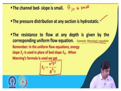
The third one is the channel bed slope is small. So, theta or S 0 is small, S0 as we have been seen in the open channel flow. The another approximation assumption is that the pressure distribution at any section is hydrostatic. This is an important one. Apart from that, the resistance to the flow at any depth is given by the corresponding uniform flow equation. This is another assumption when we are going to derive the different parameters and the properties of gradually varied flow.
