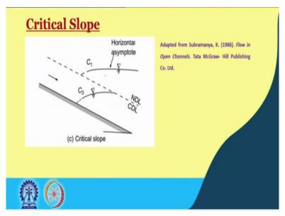
So, critical slope, so the horizontal asymptote C1 and C3, so I mean, there is much more detail to it but at undergraduate level only what we had, I mean, what I am teaching is only required, the identification of the regions, what is mild slope, what is adverse slope, what is horizontal bed.
