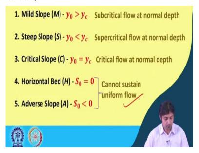
One is mild slope, that is called M, where the normal depth y0 is greater than the critical depth. So, this implies that the flow is subcritical at normal depth. See, Fr is equal to V under root gy0, if y0 is greater than critical depth, then Froude number is going to be less than 1. So, if the normal depth is greater than the critical depth, that is, subcritical flow at normal depth, then this is called mild slope.
