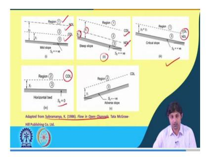
So, this is an example we have just, I mean, this diagram number 1, I mean, indicates in case of a mild slope, it shows 2 regions. What was the criteria? The normal depth, so this is normal depth and this is critical depth, so this is the line that shows, NDL corresponds to normal depth, CDL corresponds to critical depth. So, this represents a mild slope.
