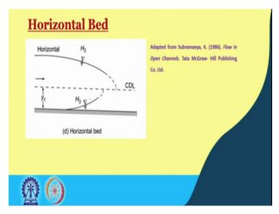
So, the horizontal bed is like this, you know, this area is H2 and this area is H3. So, if the profile is like this and if the profile is like this, which is H2, so the profile is like H2, this is H3, which is just to show you.
