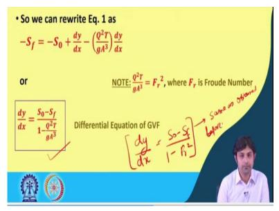
So, here T is the top width of the channel, so this equation can be rewritten as, so if we rewrite equation 1, the dH by dx was -  $S_f$ , dz by dx was minus  $S_0$ , this dy by dx is the same and this becomes Q square T by gA cube, from the previous slide and this dy by dx. Each term you have understood now, so we rearrange and we take this  $S_0$  on this side and dy by dx we take common, so let me do it for you here and then you will follow.
