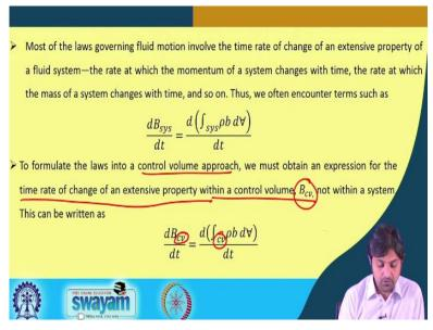
So, most of the laws governing fluid motion involve the time rate of change of an extensive property of a fluid system, the rate at which the momentum of a system changes with time, for example or the rate at which the mass of the system changes with time and so on. Thus, we often encounter terms such as dB sys dt. So, not only B system is important with that is the summation of so, B summation B sys was integral system rho b d V.
