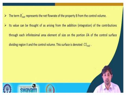
The term B out represents the net flow rate of the property B from the control volume, you see, its value can be thought of as arising from the addition of the contributions through each infinitesimal area element of size on the portion del A of the control surface dividing region 2 and control volume this surface is denoted as CS out, that is what we talked about, I was showing on the finger.
