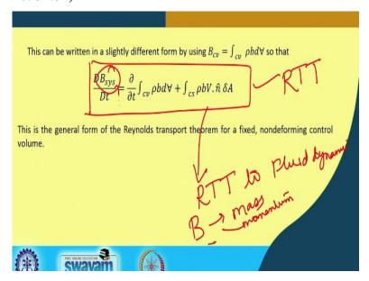
This can be written in a slightly different form by using so, that Bcv is equal to rho b dV. We can also write this in this for del del t of control volume. So, what we did? We just this, one we wrote in this format. So, now, this is the general form of Reynolds transport theorem for a fixed non deforming control volume.
