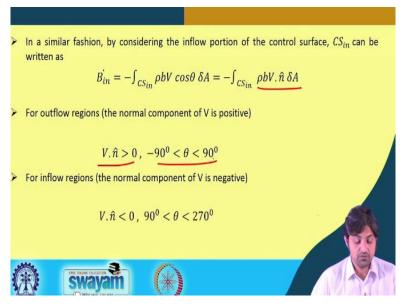
In a similar fashion, by considering the inflow portion of a control surface CS in can be written as because it was negative sign rho b V dot n cap del A. So, for outflow region just remember V dot n cap is greater than 0 and theta is between 90 degree and - 90 to 90. So, for inflow region the normal component of V is negative and for out flow region it is positive. So, V dot n cap is less than 0 and theta varies from 90 to 270 degree.
