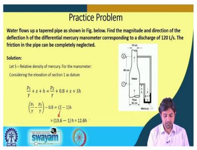
So, the problem goes like this, the water flows up a tapered pipe as shown in the figure below. Find the magnitude and direction of the deflection h of the differential mercury manometer corresponding to a discharge of 120 liters per second. The friction in the pipe can be completely neglected. The reason of neglecting the friction completely is, so that, we are able to apply, you know what, Bernoulli's equation.
