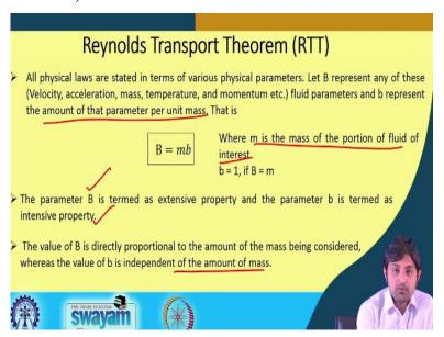
So, to start fluid dynamics, one of the most important theorems that generally is not taught in fluid mechanics is Reynolds transport theorem. So, what we are going to do, we are going to derive this Reynolds transport theorem in a little bit more detail. So, all physical laws are stated in terms of various physical parameters. So, if B represents any of these, these parameters can be velocity, acceleration, mass, temperature, momentum, anything etc.
