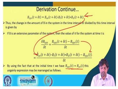
so, B system at t + delta t will be B of control volume t + delta t - B of 1 at t + delta t + B 2 at t + delta t. So, now taking you back what actually is B 1 and B 2. So, you see, this was 1, this was 2, because this has moved. Now, what earlier it was a part of B system. So, this is simply we write, B cv t + delta t - this has moved, but this has already proceeded forward so, it has come into the system of B, B system.
