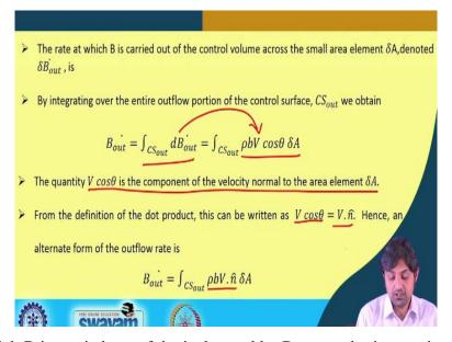
The rate at which B is carried out of the is denoted by B out so, by integrating over the entire outflow portion of the control surface we obtain B out as integral of dB out as the rho b So, we substitute this rho b V cos theta delta A. The quantity V cos theta is the component of the velocity normal to the area element delta A, from the definition of the dot product, this can be written as
