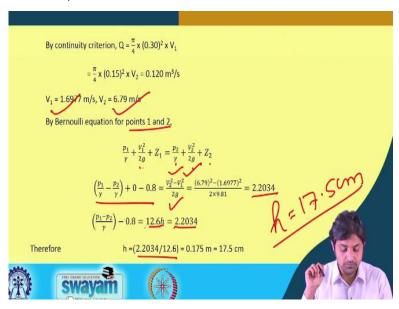
So, by continuity criterion Q is going to be you see, pi / 4 area A 1 V 1. So, V 1 we know, so, V 1 is the velocity at this section, area because this is 30 centimeters in diameter. So, pi d square / 4 into V 1 is q 1, so, d 1 pi / 4 into V 2. So, here, this is A 2, and this is V 2, this is A 1, this is V 1, so, V 1 from this method because Q is already given. What is the Q already given? 120 liters per second so, we can find V 1 and therefore, we also can find out V 2.
