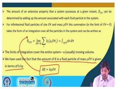
The amount of an extensive property that the system possesses at a given instant B, sys so, basis is the amount of the extensive property that a system will have at any given instant. And how that can be found out? It can be determined by adding up the amount associated with each fluid particle in the system, it is very simple. So, B system can be calculated by summing up different B s, you know, capital B, capital B of each particle.
