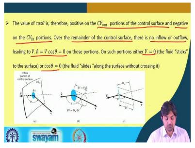
So, value of cos theta is therefore, positive on the CV out portions of the control surface and negative on the CV in portions over the remainder of the control surface, there is no inflow or outflow leading to V dot n cap is equal to 0 on those portion. On such portion either V equal to 0 or cos theta is equal to 0.
