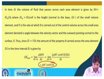
So, let us suppose, in time delta t the volume of fluid that passes across each element is given by delta ln into delta A, where delta ln is delta l cos theta, in the previous figure, is the height of the small volume of element and theta is the rate at which B is carried out of the control volume across the small element denoted, is angle between the velocity vector outward pointing normal to the surface and so theta is the, you know, the angle between the velocity and the n cap.
