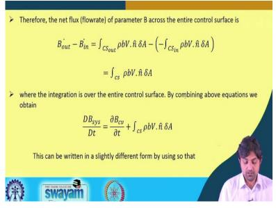
Therefore, showing the cross section in therefore the net flux of the parameter B across the entire control surface can be written as B out - B in is equal to CS out rho b V dot n cap delta A, almost the same expression just the cross sections are different or we can also write in over the entire cross section because at other places, this component is 0. There is only a contribution at outside and inside which can be taken care of from this expression.
