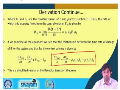
So, now putting this all together where are b 1 and rho 1 are the constant values of b and rho cross section 1. Thus, the rate at which the property flows is given by rho1 A1 V1 b1. If we combine all the equations we see that the relationship between the time rate of change of B for the system and that for the control volume is given by
