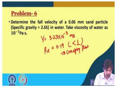
So, we have got V is equal to 3.23 into 10 to the power minus 3 meters per second and after checking the Reynolds number it came out to be 0.19 which is less than 1, therefore, creeping flow and we would have applied the terminal velocity.
