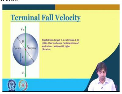
So, after this we are going to calculate the terminal fall velocity. So, if there is a sphere, you know, there is when it falls through a liquid, there is the weight acting and there is a drag force acting against its motion direction. We are going to see how we arrived at the terminal fall velocity.
