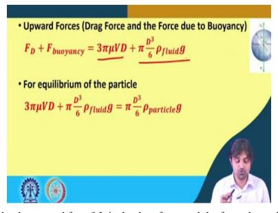
What is going to be the upward force? It is the drag force and the force due to buoyancy. So, let us say, F D is the drag force and F buoyancy is the buoyancy force. As we have already seen 2 couple of slides back, Stokes derived, the drag force as 3 pi mu V D. And the buoyancy force is
