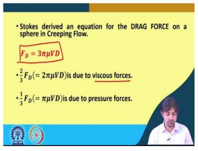
So, now Stokes derived an equation for drag force on the sphere in creeping flow. So, the derivation of the Stokes, I mean, this drag force is outside the scope. So, I am what I am going to give you is, I am going to give you directly the result. So, the drag force on the sphere is given
