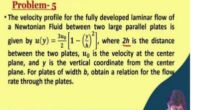
Now, we will solve one more problem, the last problem of the series of laminar flow around plates. It is a little inquisitive question. The velocity profile for the fully developed laminar flow of a Newtonian fluid between 2 large plate is given by, so, we have been given a new profile u y
