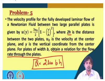
Now what we are going to do is we are going to the, so, we have to obtain a relationship for the flow rate through the plates and which we have got Q is equal to 2 u not b h for the problem that was there.
