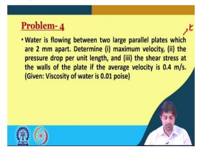
So, the question here is, water is flowing between 2 large parallel plates which are 2 millimeters apart. So, that is, means t is 2 millimeter. Determine the maximum velocity, the pressure drop per unit length, that is, dp dx and the sheer stress at the wall of the plate if the average velocity is 0.4 meters per second. And viscosity of water is given as 0.01 poise. So, to solve this, what I will go to the white screen and first write down what all things are given.
