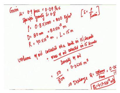
So, as always what we are going to do, we are going to write the things that are actually given. Given thing is mu is 0.9 poise or in SI unit is 0.09 Pascal seconds. We know it is specific gravity S is 0.8. Therefore, the density is given to be 0.8 and if we assume 1000 kilograms per meter cube density of water, so, the density of the fluid is 800 kilograms per meter cube, since, S is rho / rho water.
