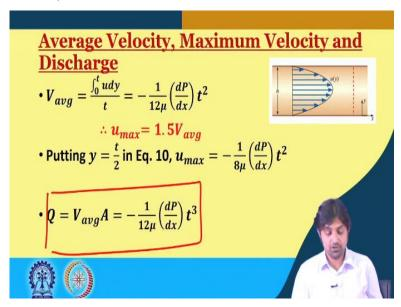
Now, repeating the same procedure of average velocity, maximum velocity and discharge. The average velocity is again given by integral 0 to t udy / t and if you put u as obtained in the last
