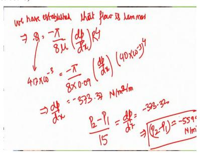
So, we are going to do the again white screen. So, we have established that flow is laminar, therefore, Q is going to be the formula that we have derived minus 8 minus pi divided by 8 mu dp dx into R to the power 4. So, Q value we already know, that is, 4.17 into 10 to the power minus 3 is equal to minus pi 8 into 0.09 dp dx into R, we know, 40 into 10 to the power minus 3 to the power 4, what we get is dp dx is equal to minus 373.32 Newton per meters square per meter.
