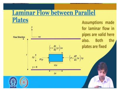
So, now we have done the laminar flow through the circular pipe. Now we are going to see the laminar flow between the parallel plates. So, this is a parallel plate. So, whatever assumptions that we have made for laminar flowing pipes are valid here also. In this case both the plates are fixed plate and this is also fixed plate. As you can observe, this is x direction and this is y direction.
