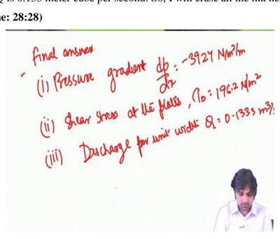
So, final answers is going to be one is the first one is pressure gradient, that was, required dP dx came out to be minus 3924 Newton per meter square per meter. Second one was shear stress at the plates, that is, tau not equal to 196.2 Newton per meter square. And the third one was
