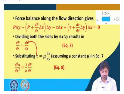
So, with this in background, we start to write the force or we do the force balance analysis along the flow direction. So, for your convenience I have made the free body diagram that is there, I have just reproduced it in the top corner. You see, P delta y, that is, force per unit length minus this one here and this again is in the negative direction tau delta x. So,
