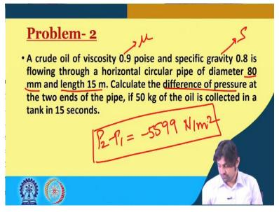
This was the difference of pressure. So, that came out to be finally and right here, P 2 - P 1 came out to be minus 5599 Newton per meters square. So, this is how we solved a detailed solution. Let me take down this ink.
