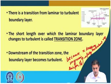
And then there is a transition from laminar to turbulent boundary layer. So, this is the transitional zone here. So, this short length over which the laminar boundary layer changes to turbulent is called the transition zone, indicated by this distance here. Now, the downstream of the transition zone, the boundary layer becomes turbulent because x keeps on increasing and therefore, Reynolds number increases leading to fully turbulent region.
