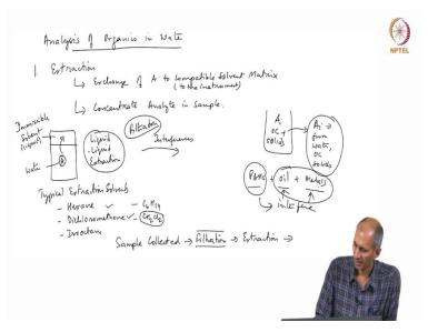
So, we look at analysis of organics in water. So, the first thing is the extraction, we look about extraction. Extraction means, we are talking about something which is at very low levels, typically, we are talking about nanogram per liter or microgram per liter that level of concentration. So, we want to pull it out. So, as if you recall the objectives of extraction are, use of compatible solvent for exchange of A to compatible solvent matrix, that is compatible means it to the instrument.
