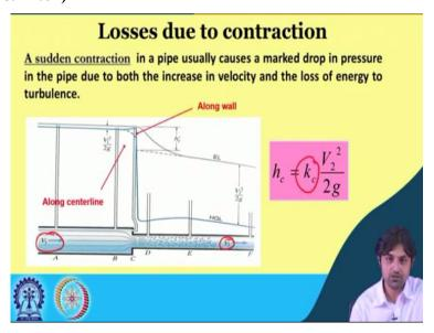
Now, let us see the loss due to contraction. A sudden contraction in a pipe usually causes a marked drop in pressure in the pipe due to both increase in the velocity and loss of energy due to turbulence, that is a well established fact, correct. So you see there is a fluid that is coming with velocity V and after the sudden contraction, the velocity changes to V2. So in this case, for a contraction, the minor head loss will be kc that we do not know yet into V2 square by 2g, not V1.
