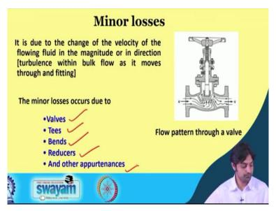
So we talk about the minor losses. We have talked much about the major losses, but now we must put our focus a little bit on the minor losses. So minor losses is due to the change of the velocity of the flowing fluid either in the magnitude or in the direction, okay. If the magnitude or the direction, any of them would change or both will change, the loss is associated with them is called minor loss in pipes. So this is a typical flow pattern through a valve, that is shown here.
