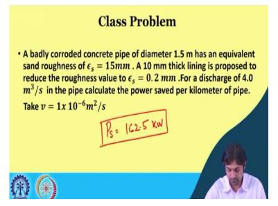
To demonstrate that, we have a problem question here, that we are going to solve now. So the question is this, a badly corroded concrete pipe of diameter 1.5 m has an equivalent sand roughness of epsilon S 15 mm. So we have already been given epsilon S. At 10 mm thick lining is proposed to reduce the roughness value to epsilon S of 0.2 mm. So a thick lining would be put, which is 10 mm long and this will bring down the roughness to 0.2 mm.
