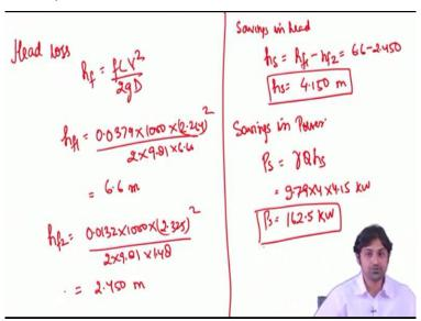
We are going to calculate head loss hf is equal to fLV square by 2gD. So before the lining was put, hf1 would be 0.0379 that was the friction factor 1, length is 1000 and velocity was 2.264 whole square divided by 2 into 9.81 into 6.60. So hf1 comes out to be 6.6 meter. Similarly, we will calculate hf2, same formula, f here now the new f was 0.0132 into 1000 into 2.325, the velocity had changed divided by 2 into 9.81 into 1.48 and this comes out to be 2.450 meter head loss.
