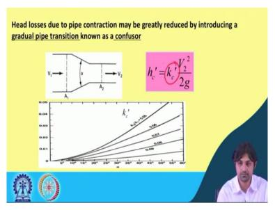
So head losses due to pipe contraction may be greatly introduced, so you see due to sudden contraction, there is going to be head losses. Now our aim as an engineer is to reduce those head losses, correct and that can be done by introducing a gradual pipe transition called as confusor. So confusors are used to introduce a gradual pipe transition, something like this. You see there is an angle alpha.
