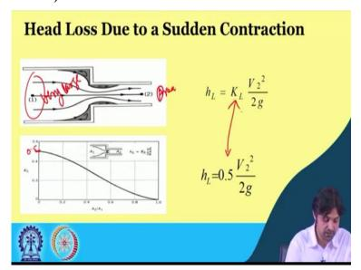
So if this is the contraction depicted by 0.2, it is a fluid at 0.1 goes a contraction and is at 0.2, we write head loss is kl into V2 square by 2g and what is this kl, kl can be found out as a function of A2 by A1. What the area 2 and area 1 is, okay, ratio of the areas, so A2 by A1. So most of the time, you would be given these values directly or a curve like this will appear, but for certain standard conditions, you are expected to know this.
