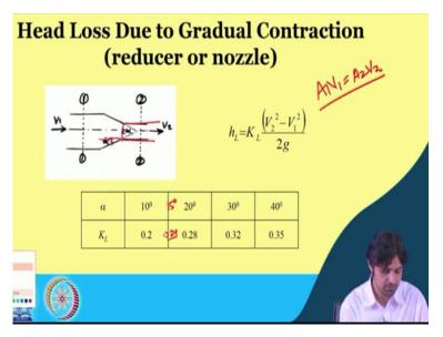
Now, in this particular case, head loss due to gradual contraction, you see, we had one equation and we can also write this in form of another thing where both V2 and V1 could be used. So kl into V2 square minus V1 square by 2g, okay in case of contraction like this, you see. This is 2 alpha and this is alpha and here also we are going to use for different alpha, we have different kls, in that case, you do not have to worry about area of 1 and area of 2.
