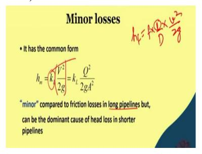
So minor losses also have a common form of this. So it is kl multiplied by V square by 2g, okay and this kl is the minor loss coefficient. In terms of Q, we can also write Q square by 2ga square. So this is minor compared to friction losses in long pipes, but can be dominant cause of head loss in shorter pipes. So if the pipe is long, because the major loss is given by f into L by D, remember 2V square by 2g, alright. So if the pipe is long, the major losses would be too much.
