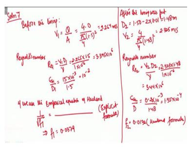
So we see, before the measure of reducing the head loss, before the lining was put, V1 is going to be Q/A, so Q was 4 meter cube per second, area is pi by 4 into 1.5 whole square. So this is going to be 2.264 meter per second, alright. For this particular case, Reynold's number is going to be, we call it Re1 as V1 D1 by nu. So V1 we have already found 2.264, diameter we know, it was 1.5 meter and nu is 1 into 10 to the power -6.
