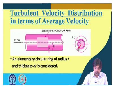
Now, we are going to talk about turbulent velocity distribution in terms of average velocity. So, there is a flow and there is an elementary circular ring here, as you can see, this is of radius R. So, we have an elementary circular ring of radius r and thickness dr which we have considered. So, radius small r and thickness dr, that is, what we have considered.
