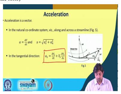
So, acceleration first thing to that you already know is a vector. In natural coordinate system, that is, we describe the acceleration along and across the stream line that we are going to see. Suppose, this is a streamline here, this in figure 5, let me take the laser pointer here. So, this is a streamline and this is a direction s and this is the velocity v direction here and this is the S
