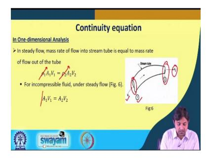
So, going to another concept, that is, continuity equation. So, in one dimensional analysis, what we see is, in a steady flow mass rate of flow into the stream tube is equal to the mass rate of flow out of the tube. So, whatever goes comes in goes out of the tube for example, in a steady flow. So, in one dimensional the continuity equation says  $\rho_1 A_1 V_1 = \rho_2 A_2 V_2$ , this is the continuity equation.
