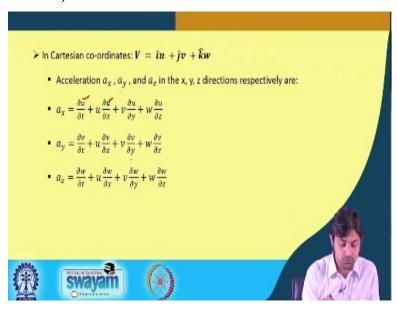
So, again in Cartesian coordinates, if we write the velocity I think, it is best again to write V as  $u\bar{t}$ , here we have written the velocity according, I mean,  $\bar{t}$ , before, it is also right, but better to. This is the normal convention. Acceleration  $a_x$ ,  $a_y$ , and  $a_z$  in the x, y and z directions respectively are. So,  $a_x$  will be written as  $\underline{\partial t}$  plus the this is local acceleration and this part is convective acceleration.
