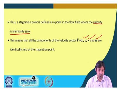
Thus, a stagnation point is defined as a point in the flow field where the velocity is, this is the key point is identically zero. This means, that the all the components of the velocity V that is u, v, and w, are identical is zero at this stagnation point. Some of it we will be going to see in today's lecture or maybe in the weeks coming forward what the stagnation point, where it can be used. Now, after all these points, we move on from the velocity description to the acceleration part.
