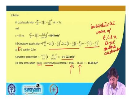
So, the solution procedure goes as like this. Local acceleration is given by  $\frac{\partial v}{\partial t}$ . So, so,  $\frac{\partial v}{\partial t}$  if you see this equation here, so, if you multiple if you do  $\frac{\partial v}{\partial t}$ , it is going to be 2t, this
