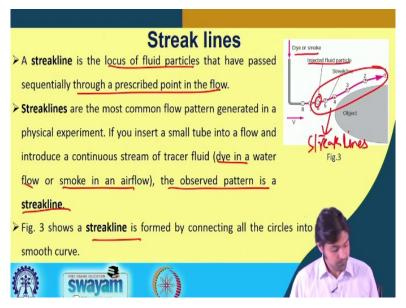
Moving to the next concept is streak lines. So, what are streak lines? So, a streak line is the locus of the fluid particles that have passed sequentially through a prescribed point in flow. So, if we start tracing the fluid particles that have passed sequentially through a prescribed point in the flow. We will explain it a little more. So, streak lines are the most common flow pattern generated in a physical experiment.
