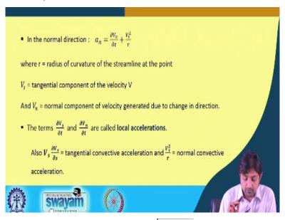
And in the normal direction it is nothing that it is  $\frac{\partial Vn}{\partial t} + \frac{V_s^2}{r}$ ,  $V_n$  and  $V_s$  are velocities in s and n direction. Here, this r is the radius of curvature of the streamline at that point. This you will we will solve some problems, maybe in the upcoming, you know, lectures.  $V_s$  is the tangential component of the velocity V. This we already talked and  $V_n$  is the normal component of the velocity generated due to change in direction.
