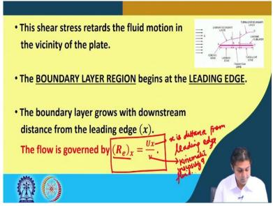
So, one of the important parameters that you have read in the fluid flow is Reynolds number. So, there is going to be a Reynolds number associated with this type of phenomenon. That is the occurrence of or the development of the boundary layer which is given by, as given here, R e at a distance x, is given by, Ux / nu. Where u is the free stream velocity here, x is the distance from the plate, a leading edge and nu is the kinematics viscosity of fluid.
