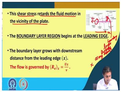
Now, the presence of this shear stress, what it does is, it retards the fluid motion in the vicinity of the plate. So, this, I mean, in the existence of the velocity gradient will induce shear stress and that is going to slow down the fluid motion near the plate. And the boundary region therefore, will start occurring at the leading edge because that is the first point where the velocity is zero. And, as soon as, we go over and above it there will be certain velocity.
