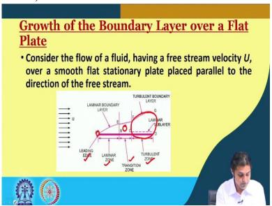
Now, after this brief introduction, we will talk about how the boundary layer grows over a flat plate. This is the most simplified object that you think of is a flat plate above when the flow will passed over it how the boundary layer will grow above that. So, to do that we have to consider the flow of the fluid having free stream velocity U and that happens over a smooth flat stationary plate placed parallel to the direction of the free stream. So, something like this.
