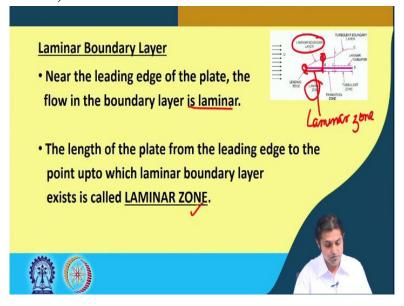
Now, what is laminar boundary layer? We are going to continue, this is the laminar zone, so we are going to concentrate on that. Near the leading edge of the plate the flow in the boundary layer is laminar. This is important to note. And the length of the plate from the leading edge to the point upto which laminar boundary layer exists is called laminar zone. So, this is the leading
