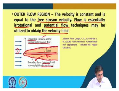
Then the second region is called the outer flow region. The velocity is constant here and is equal to the free stream velocity. As I told you in the initial slides that above this boundary layer the velocity will not be effected, it will be the same as this free stream velocity that was the flow was coming with whatever velocity it had before the same will be maintained above this boundary layer.
