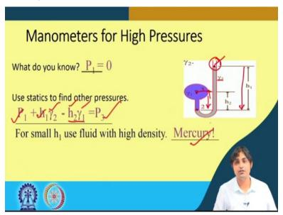
So, what do we know, we know that pressure at 1 is 0 because this is exposed to atmosphere. We have to use statics to find the other pressures here. So, P1 so, if the pressure at here it is  $p_1 + h_1 \gamma_2$  because the same fluid the pressure is increasing as direction multiplied by the density, this is the pressure  $h_1 \gamma_2$ . So, now we are going up by how much,  $h_2$ , if you want to go to the center we are going up so  $-h_2 \gamma_1$  should be equal to  $p_3$ .
