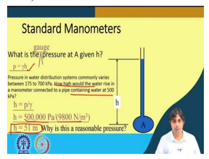
For standard manometers. What is the pressure? So how it works is very simple example. So, what is if we are asked, what is the pressure at A given the height, more importantly we should mention what is the gauge pressure. Because gauge means we are not counting the atmospheric
