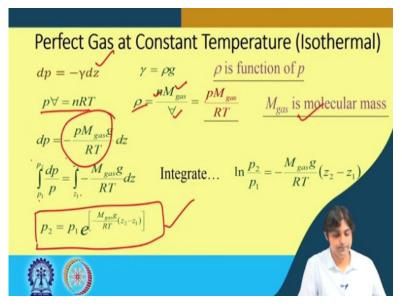
Now, we are going to do perfect gas at constant temperature that is isothermal process, we start with the same old equation  $d\mathbf{p} = -\gamma d\mathbf{z}$ . And where gamma is  $\gamma = \rho \mathbf{g}$  where the  $\rho$  is a function of P. So, because in gas it is PV = nRT that is the thumb rule for isothermal. So,  $\rho$  can be written as  $n*M_{gas}/V$  or in other terms we can write it as  $pM_{gas}/RT$ ,  $M_{gas}$  is the molecular mass which we have seen in lecture number 1.
