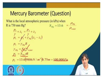
So, we have seen this equation piezometric head is constant. So, we can also write let me erase this one. P1 is  $P_1 = P_2 + \gamma_{Hg}(Z_2 - Z_1)$ . We are putting this piezometric head equation between point 1 and point 2 and we want to calculate the pressure at p1. p 2 atmospheric pressure so, atmospheric pressure we assume gauge pressure that can be assumed 0 that you have read in
