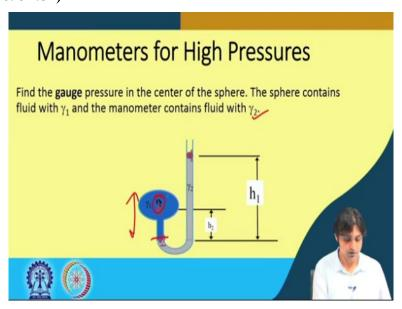
Another example for a differential you know, manometer. So, find the gauge pressure in the center of the sphere. So, this is not a differential. So, we are we are going to measure the high
