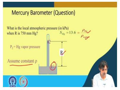
So, this is the barometer. This is the principle of working of barometers. Now, a simple question is, what is the local atmospheric pressure when R is 750 millimeters of Hg. This is R we are just going to see we have given the  $\frac{\rho_{Hg}}{\rho_W}$ =13.6 then we have assumed incompressible fluid constant  $\rho$ , we are going to see how it works. So, this is point 1 here and this is point 2 here.
