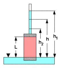
Total head h in standpipe of area a is allowed to fall. Hydraulic gradient varies with time. Heads  $h_1$  and  $h_2$  are measured at times  $t_1$  and  $t_2$ . At any time t, flow through the soil sample of cross-sectional area A is
