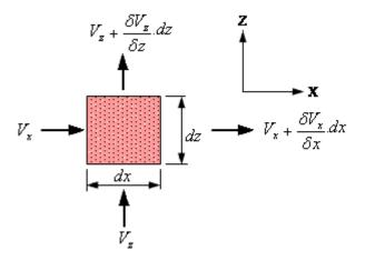
A rectangular soil element is shown with dimensions dx and dz in the plane, and thickness dy perpendicuar to this plane. Consider planar flow into the rectangular soil element.
