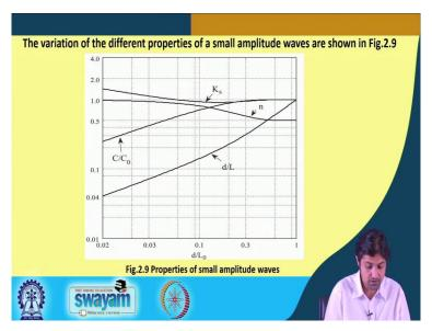
So, the variation of different properties of a small amplitude waves are shown in this figure you do not need to pay too much attention just we have plotted d by L C by C not k s and n which you already know chaos is the shoaling coefficient.
