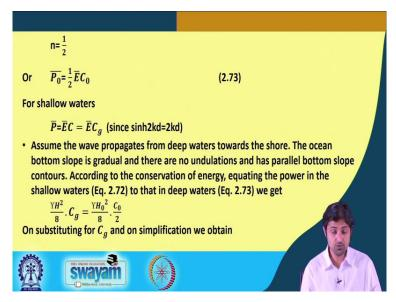
n = half so, power is going to be half into C not for shallow water it will e into CG because CG is C only if you assume that the wave propagates from deep water towards the shore and the ocean bottom slope is gradual and there are no undulations and as parallel bottom slope because, you see the wave power is going to be conserved if the wave moves from 1 depth to the other. Because you see this if there is no loss, it is average energy flux per unit wave crest rate.
