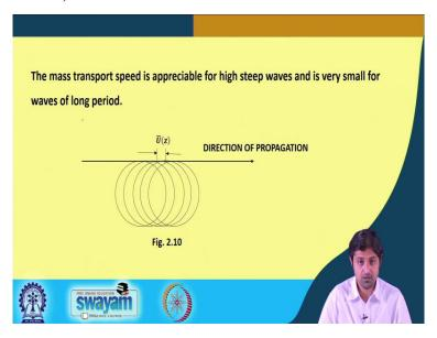
So, the mass transport speed is appreciable for high steep waves and very small for waves of long period you can see this equation. So, if it is a long wave, the mass transport is very less because, so if period is long the length is long. It is the high steep wave which means which is directly proportional to h squared. So, the mass transport will be high for long the higher waves.
