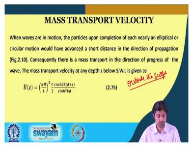
So, this is the last topic the derivation is outside the scope, but what you must understand is that when waves are in motion, the particles upon completion of each nearly an elliptical or circular motion would have an advanced a short distance in the direction of propagation of waves, you can check it from those equations as well. Therefore, if they move ahead that means that the
