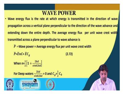
So, now we have studied wave energy it is very obvious that we study wave power wave energy flux is the rate at which energy is transmitted in the direction of wave propagation across a vertical plane perpendicular to the direction of wave advance and extending down the entire. So, the average energy flux per unit wave crest with transmitted across the plane perpendicular to the wave advances is wave power. And it is given as e into CG.
