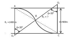
In given Figure, A and C are the points of tangencies and B is the point of reverse curvature (PRC). The distance between the lines V = 469 m
