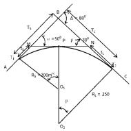
Given-  $R_S = 200$  m,  $R_L = 250$  m,  $\Delta = 80^0$ , chainage of the intersection point = 1504.80 m, and  $\angle$  BMN =  $\alpha = 50^0$ .
