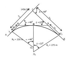
Bearing of AC is  $59^0$  30', of CB is  $127^0$  30', and of MN is  $105^0$  30'. Chainage of the intersection point is 1456.5 m. Radius of the first arc (Rs) is 220 m, and that of second arc (R<sub>L</sub>) is 275 m. Let D be the point on the line MN.
