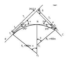
In above Figure,  $R_L = 600$  m,  $R_S = 400$ m,  $\angle$  BEF =  $140^0$ ,  $\angle$  EFC =  $140^0$ , Chainage of the intersection point A = 3415 m.
