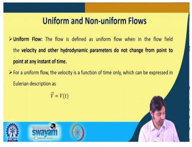
So, we have seen steady and unsteady flow. Now, we are going to see uniform and non uniform flows, the definition of the uniform and non uniform flow. Uniform flow, the flow is defined as uniform flow when the flow field that is the velocity and the other hydrodynamic parameters do not change from point to point. So, in a steady flow it was not changing with respect to time, here, these properties should not be changing with respect to the space at any instant of time.
