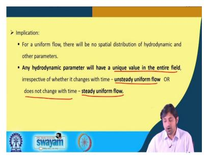
Implications for a uniform flow; there will be no spatial distribution of hydrodynamic and other parameters, as we told, because the parameters really does not depend upon the location. Any hydrodynamic parameter will have a unique value in the entire field, irrespective of whether it changes with time. Therefore, now, we have two parameters here is space and time, time was with if something depends upon time, it will be unsteady, if something does not depend upon time it will be steady.
