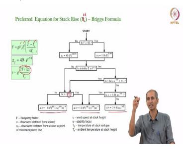
Something the velocity of the stack and the temperature is the formula that people have derived, so I am not going through this, we will just give you an idea of this several things. This is a preferred equation for calculating stack rise, Hs is delta h not Hs. So you are calculating all these
