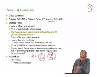
we will come back to that in a minute, so the last thing we have is what is called as emission rate, this is the most important parameter without this there is no Gaussian dispersion model, this is emission. You must know what the emission rate? So emission rate in general there are different types of way in which we estimate emission rate for different processes. But when you have things like point sources.
