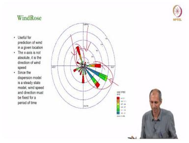
Typically, what people use is Windrose for average wind directions. This windrose is a compilation of wind speed in a given area. This is an example of how wind patterns in a given location, for example, this could be a windrose for a given city for a day, for a month, for a year. So this is an average windrose. So what the way this is read is, for example, there are different representations, you can go and search for windrose and it will give you different kinds of representation.
