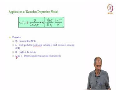
So these are the parameters that we are interested in, so in order to calculate  $\rho_{A1}(x,y,z,H)$ , four things are important: Q is emission rate,  $u_x$  is wind speed at the stack height. So this is the wind speed at stack height. So What we mean by that is, we will come off to each point separately. H is the height of the stack and  $\sigma_v$  and  $\sigma_z$  in y and z directions.
