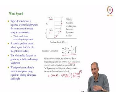
So the first parameter, wind speed. You need to calculate wind speed at the stack height, so stack height may be 50 meters, 50feet, 100feet or whatever it is. There is also the observation that typically wind speed if you look at wind speed. If I say I am looking at a stack in some place in Chennai, then what is the wind speed? Then you'll go to the nearest wind measurement? There is an anemometer in an airport or some place, somebody would have measured some value.
