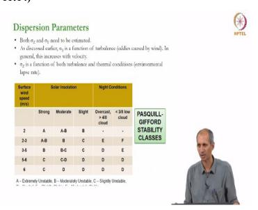
All these are only tools for doing it. The next thing the dispersion parameters sigma z and sigma y need to be estimated. So these are caused by two things one is eddies caused by turbulence in both directions y and z directions and the thermal stability class. So a very old classification in the system of what is called a stability classes. This is very old 50's or 60's by PASQUILL and GIFFORD popularly known as this.
