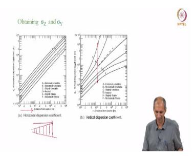
Then I use these charts, which is also given by them to give the value of sigma y and sigma z, so sigma y does not change a whole lot. So you can see stability A to B are very close to each other. It is on the y axis; x axis is the distance from the source. This exactly gives you the plume shape, as the distance from the source is increasing along the x axis, you see that the sigma y is increasing which means the plume is increasing if we are looking at sigma y is increasing.
