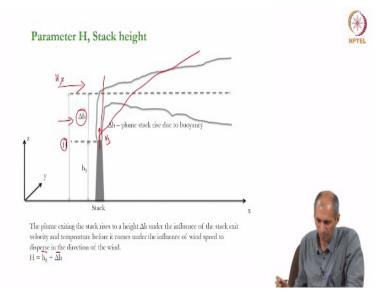
So the third the last parameter that we have is a parameter H ok, so this is simply as we see in this case it is not just the height of the stack, it is the height of this center point where you have the highest concentration. Which means that will happen for these things will happen. For example, in this example we are seeing that this plume is getting out and is going up to a certain height before it starts turning and going in the direction of the wind, why does this happen?
