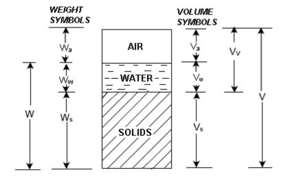
The soil model is given dimensional values for the solid, water and air components.
