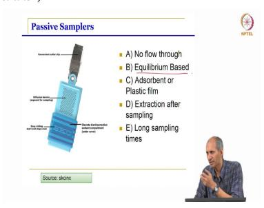
So, this is the other type of samples. This is something called as passive sampler, this is a new thing, and not a standard method, this is still under development. So, this is an equilibrium based sampler, which means that in all the other things what we have done is we take a sample of air, we know what's the volume of air and we extract whatever is there and that we exactly get concentration mass by volume.
