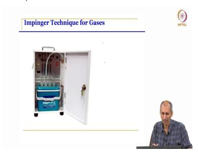
So normally the technique that is used for the priority gases, SO2, NO2, you can impinge and collect it in a solution and measure it as a chemical method for doing it. It is all there in the standard methods. The other option is you have some equipment which does that there is equipment which use UV fluorescence and things like that, ok. So, it is all there in this, just go and read it, I think there is nothing extra that I can.
