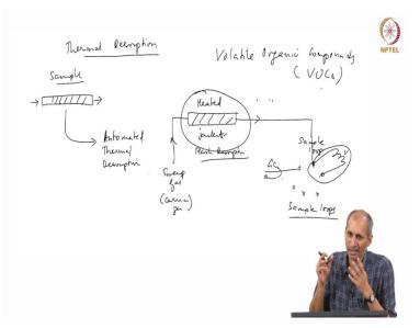
So, while coming back to our thermal desorption what is done is the following. So, you take your sample in a tube, you attach it to a pump in the usual way and then this tube is brought to what is called now called as an automated thermal desorption unit. It is an accessory to a GC, it is kept before a GC. It doesn't have to be a GC, it can be anything, any analytical instrument it is an accessory before analytical instrument the processing accessory.
