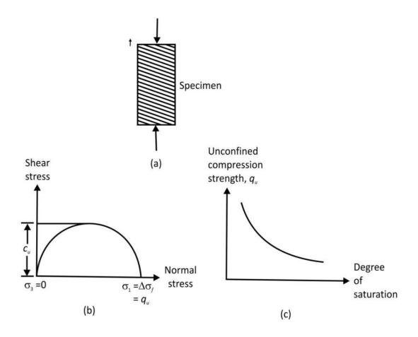
Unconfined compression test: (a) soil specimen; (b) Mohr's circle for the test; (c) variation of qu with the degree of saturation
