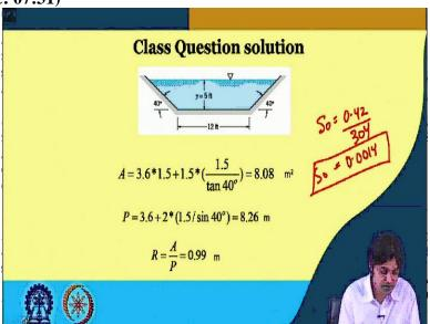
So, we start. So, this is the figure, so area is going to be, you know, 3.6 into 1.5, so this is the, this area, because we have converted it already into meter square, plus this is half base into height and half base into height, so when you add this, this will become one into base into height, base is half, so height is, sorry, height is half and base is, so it becomes 1.5 divided by tan 40 and this will come out to be 8.08 meter square.
