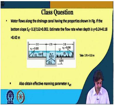
So, you see, we have found out the all the questions, I mean, all the things that we wanted to. So, we go to solve another question now. It says that, water flows in a channel shown in figure below, this is the figure, at a rate Q is equal to, no, so water flows along a drainage channel having the properties shown in this figure. If, the bottom slope S 0 is equal to 0.3. So, we have already been given S 0. Estimate the flow rate when depth is y 0, I mean, depth is 0.24 plus 0.18 that is 0.42.
