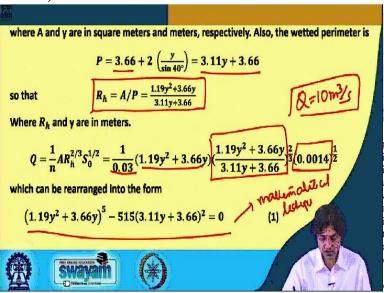
plus 2 multiplied by, because this is one and plus 1, so this will be, if this is y this is going to be  $y / \sin 40$ . And this is what we have done in terms of y, we have also written the parameter 3.11 y + 3.66. So, the hydraulic radius will come, area by parameter that is 1.19 y square + 3.66 y divided by the parameter. The discharge according to the Manning's is given by, 1 by n, n is given as 0.03.
