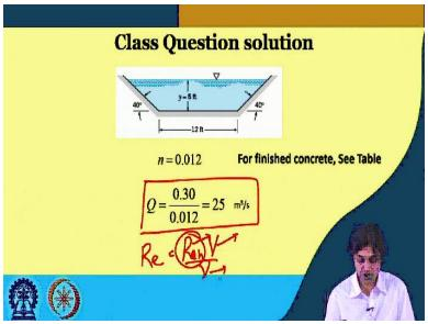
But, n for finished concrete is 0.012, so the Q comes out to be 25 meter cube per second, approximately. So, we have calculated. We have used the Manning's equation and calculated area, we have calculated parameter, we have calculated the discharge Q for this channel, for a uniform flow condition. So, the next question says we have to calculate the Reynolds number. So, Reynolds number is given by Reynolds number h V / nu and this is the hydraulic radius.
