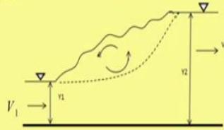
$$\text{Initial Froude number } F_1 = \frac{V_1}{\sqrt{gy_1}} = \frac{10.0}{\sqrt{9.81 \times 0.25}} = 6.386$$
