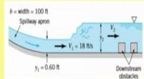
We obtain  $V_2$  by equating the flow rate
