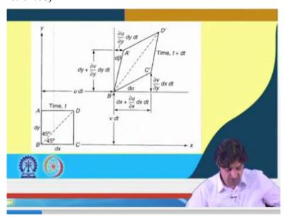
If you remember this figure, AB and BC, you know, so the 2 dimensional shear strain is the average decrease of the angle between the side AB and BC. So, we can define, this is the average, so that is the 2 dimensional shear strain is average of, so  $\frac{1}{2} \left( \frac{d\alpha}{dt} + \frac{d\beta}{dt} \right)$ , because that
