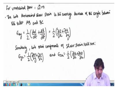
So, you know already for irrotational flow, omega is actually 0, because that is in; that is the vorticity vector should be 0. Now, the 2 dimensional shear strain is the average decrease of the angle between the sides AB and BC, in this figure.
