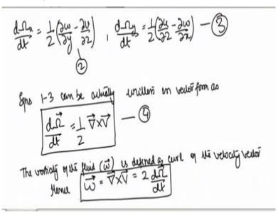
And also the rotation, what is rotation, how this angle is rotated, so we started from basics and until now we have derived that the rotation per unit time is given in a vector form as this, that was where we concluded in the last lecture. So, we will continue now, so this is, so there is a term called the vorticity. So, the vorticity of the fluid, this is actually the rate of rotation, this above equation, which let us say, I will name it as equation number 4.
