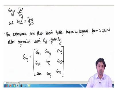
Similarly, along y and z direction, epsilon yy can be written as del v by del y and epsilon zz can be written as del w by del z. So, the extensional and shear strain rates, taken as together, form a second order symmetric tensor epsilon ij given by; so, epsilon ij, see, this is quite important, so we have actually found out the values in terms of del v, del v del x, del v del y, del v del z, another similar components.
