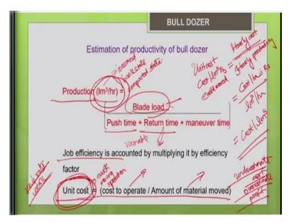
So, for that you need to know unit cost is nothing but cost per loose meter cube. Say I am going to find it in the loosen state cost per meter cube of earth moved, I need to calculate. It is nothing but your hourly cost associated with the machine divided by the hourly productivity. If we know these 2 data I can calculate. So, by now you should be knowing how to estimate the cost associated with the machine.
