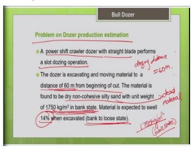
In this problem we are going to estimate the productivity of this power shift crawler dozer. So, power shift, so it is automatic gear change, so you can assume the maneuver time. The dozer is with a straight blade, it performs a slot dozing operation. The slot dozing operation you know that we adopt it, so that we can reduce the end spillage and you can increase the productivity of the bulldozer.
