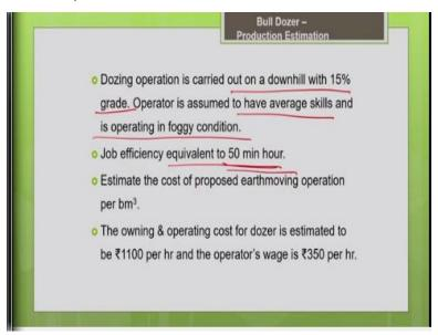
Dozing operation is carried out on a downhill, so with a 15% grade. So, your machine is moving down the slope, so this is obviously going to help you in enhancement of the productivity the operator is assumed to have average skill, not excellent skill, he is just having average skill. And it is our machine is operated in foggy condition, so it means a visibility is going to be poor. And the job efficiency is given is 15 minutes hour, that means the machine is working for 15 minutes in one hour.
