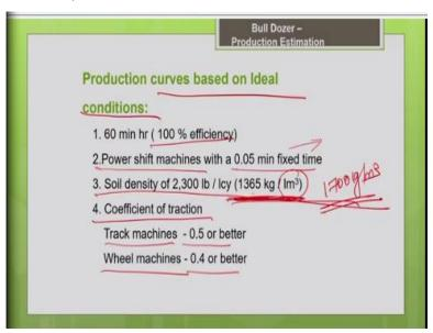
So, as I told you these production curves are drawn based upon ideal conditions. What are all ideal conditions? It is drawn assuming 100% job efficiency, that means your machine is going to work for 60 minutes in a hour, so that is what is the assumption. But in your real project site, your machine will be working just for 30 minutes or 45 minutes or 50 minutes. So, you have to apply the correction factor accordingly.
