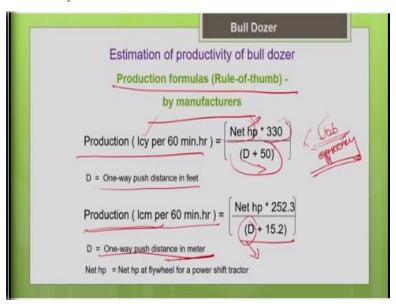
So, there are some thumb rules available provided with a equipment manufacturers. So, if you know the horsepower of the tractor and if you know the dozing distance, one-way push distance you can directly estimate the productivity of the bulldozer, these are thumb rules. It is nothing but your say net horsepower multiplied by 330 divided by D + 50, D is your one-way push distance or dozing distance in feet.
