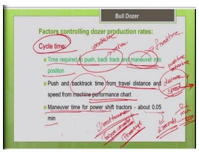
One is either you can have direct transmission or you can have this torque converter mode or power shift. Direct transmission is nothing but manual gear change. So, the operator has to manually change the gear depending upon the load conditions. Here the torque converter it will automatically match the engine output according to the load condition, you need not change the gear manually in the torque converter, it is automatic gear change.
