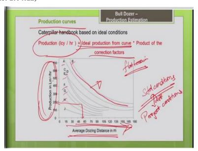
So, there is also another approach to determine the productivity. So, with the help of production curves, say some of the equipment manufacturers they do supply these production curves for the different models which they have manufactured. So, from this production curves, this just show some sample curves and schematic diagram, these are not very accurate, I am just trying to show the trend of the production curves and the application the production curves.
