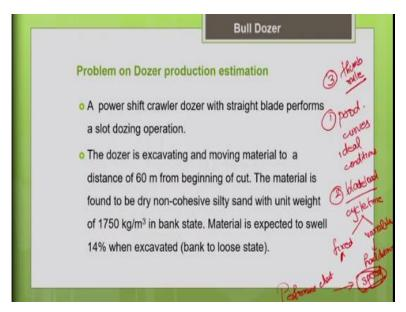
So, using production curves, which are drawn for the ideal conditions? So, we choose the value from the corresponding production curve which is supplied by the manufacturer. And apply the correction factors according to the project conditions and find the actual productivity for the project conditions, that is one way. The other method we learnt is, so we need to estimate the blade load, we need to know the blade capacity and then we need to determine the cycle time.
