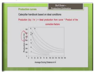
I hope you remember the sample of production curves which I have shown you earlier. So, if you know that dozing distance I can find the production curves. So, in this case the dozing distance is given as 60 meters. So, corresponding to your dozing distance if you know the model you can calculate the productivity. So, these curves are just some sample curves.
