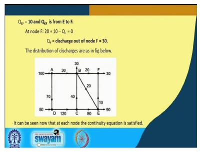
Welcome back to the next lecture. So, last lecture we finished with the equation of continuity and solving a very simple problem for a pipe flow where the discharges were given. So, we have seen it the equation of continuity A 1 V 1 = A 2 V 2.
