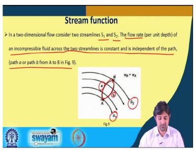
Now, stream function, what actually is a stream function? So, in a 2d flow or a 2 dimensional flow, this type of flow considers two stream lines S1 and S2. The flow rate per unit depth of an incompressible fluid across two stream lines is constant and independent of the path. So,
