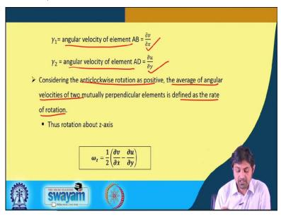
Gamma1 here, is angular velocity of element AB which is equal to del v del x. Gamma 2 is angular velocity of element ad, that is, del u del y. We can go back to this slide here, you see, del v del x and this is del u del y as we have written. Considering the anti clockwise rotation as positive, the average of the angular velocities of the 2 mutually perpendicular elements is defined as rate of rotation.
