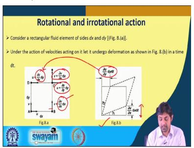
Now, talk about rotational and irrotational action. If we consider, a rectangular fluid element of side dx and dy, as in this figure you see, this is point A, this is point B, here, point A, point B, and this is dx, this is the distance, I mean, this is the distance of, you know, the side, dx and this is the dy. This is a fluid particle. Under the action of velocities, for example, here there is a velocity A, at A it is u and at in the in the x direction and V in the y direction.
