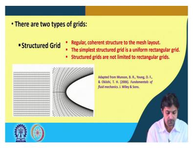
So, we talked about grids so, there are actually 2 types of grids. One is a structured grid and the structured grid means the grids are regular and coherent structure to the mesh layer. These are the simplest the structured grid and they are generally uniform rectangular grid those are called the structured grids. So, the structured grids look like this one here. So, you see they have a uniform rectangular grid. So these all the small shapes are rectangular.
