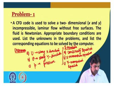
So, there is one question which I would want to know, solve solver discuss. So there is a CFD code which is used to solve a 2 dimensional in 2 dimension X and Y incompressible laminar flow without free surfaces. The fluid is Newtonian. So appropriate boundary conditions are used. So the question here is now lists the unknowns in the problem and list the corresponding equations to be solved by the computer.
