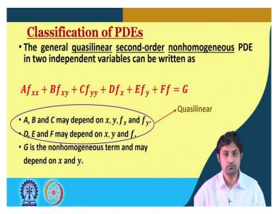
So, going to take a slight detour, because it is important that we try to remember what the classification of partial differential equations look like. So, they are general quasilinear second order non-homogeneous partial differential equation in 2 independent variables can be written as Af xx + Bf xy + Cf yy + Df x + Ef y + Ff = G, this is a general quasilinear second order we have x x, x y and y y that is second order non-homogeneous or partial differential equation.
