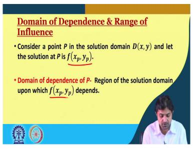
Now going to domain of dependence and range of influence. So, if you consider a point P in the solution domain, so, there is a point in the domain P and let the solution at P if we assume that the solution at that particular point P is f(x p, y p) we assume that then the domain of dependence of P is the region of solution domain upon which f(x p, y p) depends.
