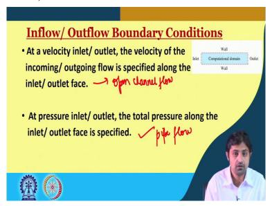
No not talking about the inflow and the outflow boundary conditions. So, you see this is inlet this is outlet. So, the here from here the inflow will be there, and from here out flow will be there. In means coming in and out means going out. So, at a velocity inlet or outlet the velocity of the incoming or outgoing flow specified along the inlet outlet phase at pressure inlet and outlet the total pressure along the inlet and outlet phase specified.
