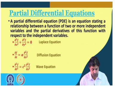
So, now, we come to the, in the solver stage we come to we have this way we have mentioned about the boundary condition and now we come to discuss about the partial differential equations. So, partial differential equation PDE is an equation stating a relationship between a function of two or more independent variables and the partial derivatives of this function with respect to the independent variable. So, this is the definition of partial differential equation.
