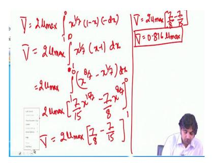
So, using the, we write V bar is equal to 2 u max integral x to the power 1 by 7 one minus x minus dx. So, that is from 1 to 0. So, it will be 2 u max integral 0 to 1 x to the power 1 by 7 x minus 1 dx or 2 u max x to the power 8 by 7 minus x to the power 7 dx, that is, 1 to 0. These limits have to be checked 1 to 0. So, it was 1 to 0, 1 to 0, 1 to 0.
