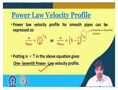
Now, about the power law velocity profile, a little bit on that. So, the power law velocity profile for smooth pipes can be expressed as, it is, u by u max can be written as y by R to the power 1 by n. This is the power law velocity that was given or we can always write in terms of R because y is, y is R minus small r and that you substitute here, you will end up in this equation. So, this 1/n
