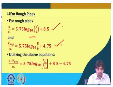
Now, we did it for smooth pipes. Now, for rough pipes, we have an equation and we also obtained V average by u star. We do the same procedure, we subtract this equation, we subtract this equation from this equation. So, this minus this and utilizing the above equation, we get u minus V average by u star. So, we have got y by k divided by R by k plus 8.5 minus 4.75
