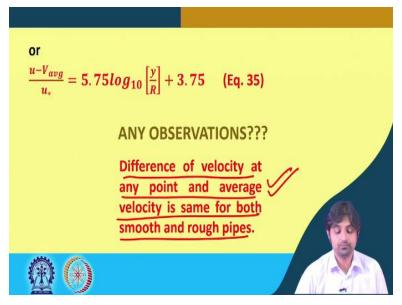
Or we can simply get u minus V average by u star is equal to 5.75 log to the base 10 y by R plus 3.75. Is there any observation? If you see for either for smooth or for rough this difference came out to be the same. So, the observation is the difference of velocity at any point and average velocity is same for both smooth and rough pipes. This is important to know that.
