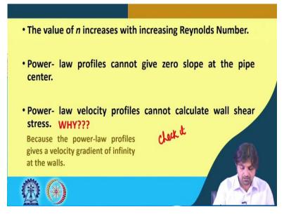
The value of n will increase with increasing Reynolds number. Power law velocity profiles cannot give 0 slope at the pipe center. So, power law of velocity profiles also cannot calculate the wall shear stress. Why? Because the power law profiles gives a velocity gradient of infinity at the walls. That you can try, by substituting r is equal to, small r is equal to capital R. You can check it check it at.
