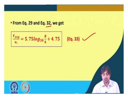
So, what is this? This is the average velocity divided by the frictional velocity for the turbulent pipe flow case.
