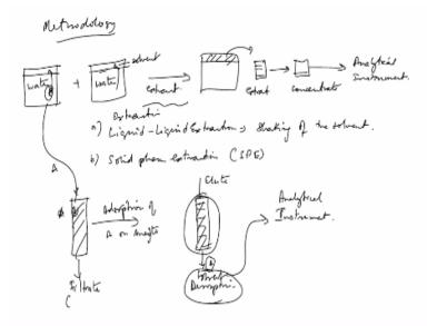
So you have a water sample. Now you add a solvent. You extract, then you transfer the extract into another bottle and then you concentrate it further and the analytical instrument. So these extraction methodology you can have various ways of doing it. One method of extraction is called as a liquid-liquid extraction where you add a solvent and then shake it and then you keep shaking it.
