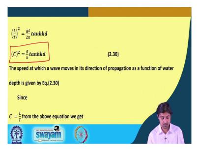
So, but is substituting since sigma and k in terms we get L by T whole square = gL by 2 pi into tan h k d or C squared =, because it can be written as C square = g by k into tan h k d. So, the speed at which a wave moves in the direction of propagation as a function of what a depth can be given by equation. Earlier we obtained the velocity potential at constant depth but now we have found out the speed of the wave as a function of water depth.
