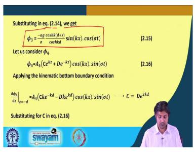
And same procedure is repeated for the dynamic free surface boundary condition and we get for phi 3 at term like this, you understand same procedure. So phi 3 we get - ag by sigma cos h k d + z similarly, we get phi 3. And same procedure we do for phi 4, for obtaining the values.
