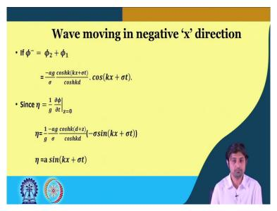
Now, if there is a wave that is moving in x direction, then we can simply write the velocity potential phi - = phi 2 + phi 1 not - phi 1 and then we will get nothing but with -  $\sin$  - ag by sigma  $\cos h k x$  sigma k x + sigma t into  $\cos h k d$ . So, what you do is you do  $k = \sin h k d$  so, instead of  $k = \sin h k d$  sigma t becomes  $\cos k x$  + sigma t. So, this is a different waveform. So, in this case, since a eta is
