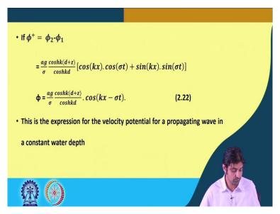
More important is this term so phi 1 we get is - ag by sigma  $\cos h k d + z$  if you remember, phi 2 and phi 4 was positive with a positive sign phi 4 and phi 1 was with the negative sign after the derivation. Now you remember I said that the total velocity potential will be the summation of the two terms. So our velocity potential is going to be phi 2 - phi 1, or also in terms of phi 3 and phi 4 also so this becomes, so if you add to velocity potential, this was you know, phi 2.
