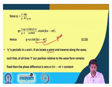
Now, because we have got the velocity potential we can finally write the term for eta, we are going to check so, eta can be return as so, 1 by g ag by sigma, so, del phi del t at z = 0 will come out to be this one. So, ag can be return as so, if you just g and g will cancel sigma and sigma will cancel. So, at z = 0, this will also get canceled. So, simply we left with n = a sine k x - sigma t.
