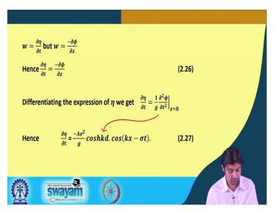
W = del eta del t but w also equal to - del phi del z in form of velocity potential hence del eta by del t equal to - del phi del z we know the velocity potential we know the equation of a eta, if we do the differentiation of a eta we get del t = one. So, if you do the differentiating the expression of eta, what do we get? Del eta by del t = 1 by g you remember, that term headset = 0 1 by g del square phi by del t square.
