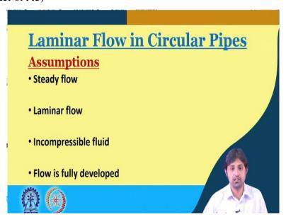
So, now laminar flow in circular pipes, so, after dealing telling you the basics of how to define the, you know, how to define and find what laminar and turbulent flow is, we are going to see some of the properties of laminar flow in circular pipes. So, for deriving anything there are certain assumptions first that we have to take. We have to assume steady flow, what does this assumption of steady flow mean, that the situation or the condition is not dependent on time.
