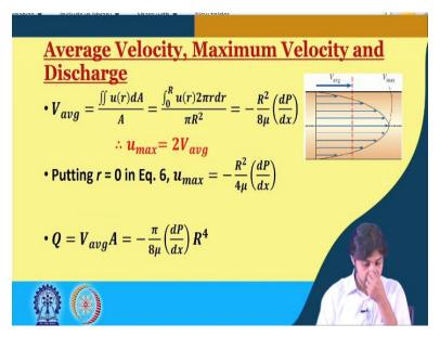
Now, what is being what will be the average velocity, maximum velocity and the discharge in this type of flow. So, the average velocity will be integration of velocity with a small area divided by entire area, this is the definition of average velocity. And if you put, u r as what we have obtained from the last slide and if you assume that small element it is the area will be 2 pi r dr, correct.
