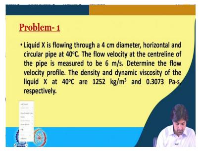
So, now we are going to see the first problem from the laminar flow. So, the problem is, there is a liquid X which is flowing through a 4 centimeter diameter, horizontal and a circular pipe at 40 degree centigrade. This is what we have done before. The flow velocity at the centerline of the pipe is measured to be 6 meter per second. So, basically what this says we have measured the centerline velocity of the pipe.
