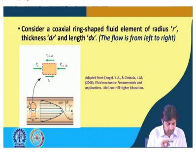
Now, after going through the assumptions, we will consider a coaxial ring shaped fluid element of radius 'r' whose thickness is 'dr' and length is 'dx' and the flow is from left to right. As I said,
