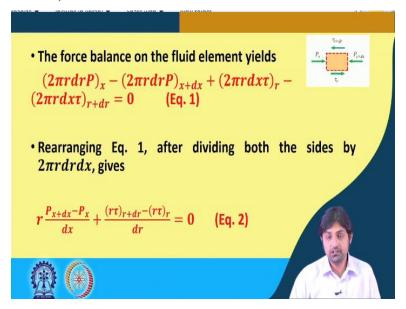
So, we have kept this figure for the forces in the right hand side. So, if you see, there will be pressure forces acting P x from the left, P x + P pressure force are at x + dx from the right and then there will be shear forces acting here, in this direction and there will be shear forces acting at Tr + dr, you know, and if we apply the force balance, so,
