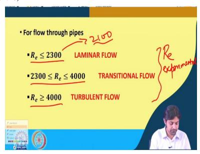
For example, for flow through pipes, if the Reynolds number is less than 2300, we consider the flow as laminar flow, important to remember. So, if you are given, the pipe diameter, the flow velocity, you can easily tell if the flow is laminar or turbulent. What you can do is, you can calculate Reynolds number as VD by nu, this is known, this is told and D is also told. So, you can calculate Reynolds number. For Reynolds number between 2300 and 4000 the flow is transitional.
