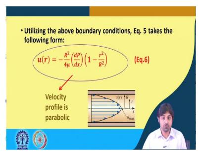
So, if we utilize the above boundary conditions, equation 5 will take the following form. So, C 1 and C 2 will be eliminated and we will have u as a function of r will be given as
