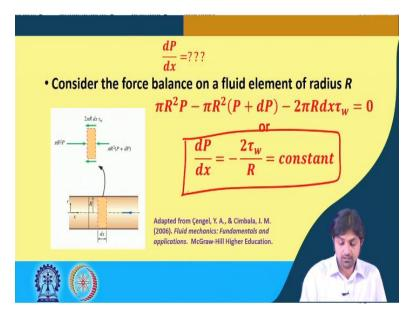
So, now what is dP dx? So, to find dP dx, we have to consider the force balance on fluid element of radius R. So, we consider a fluid element of radius R, it is quite simple, their pressure here is P. So, it becomes pi R square P, this force and this force is pi R square P + dP and the same thing is there is the shear stress acting here. So, this is the tau w. So, almost the same type of equation is there, pi R square P - pi R square P + dP force balance - 2 pi Rdx tau w.
