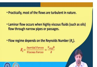
What happens in nature practically most of the flows in the nature are at turbulent, most of flow, we rarely find laminar flow. One real-life example of a laminar flow actually occurs in the our blood system. So, in the veins and in the arteries the flow can be laminar, actually it is laminar. We will tell you the reasons why later. Laminar flow can also occur when a highly viscous fluids, such as, oil flow through a narrow pipe or passages.
