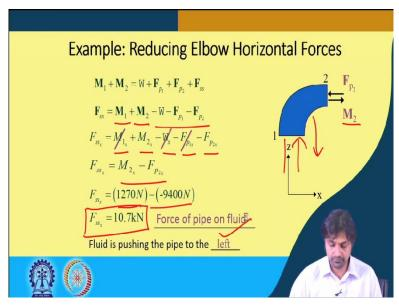
Now, it is important to find out the horizontal forces. This is what we have is, we have calculated the vertical forces. So, the same M 1 + M 2 = W + F p1 + F p2 + F ss. So, F ss is going to be M 1 + M 2 - W - F p1 - F p2 or F ss x, in x direction, because there are 2 components, it will be M1 x + M 2 x - W x - F p1 x - F p2 x.
