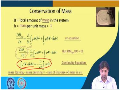
So, now conservation of mass, how can we apply, what we have learned in Reynolds transport theorem to the conservation of mass. So, B is total amount of mass in the system, when we do the conservation of mass B which we saw in Reynolds transport theorem is the total amount of mass in the system and b will be mass per unit mass which is equal to 1. So, we have determined B and b for the conservation of mass. So, B is M, capital B is M and small b is 1.
