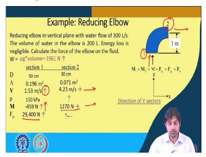
An example we are going to see is the reducing elbow using this equation, we have seen this equation already in the last slide, this is sectional 1, this is section 2, the distance between this
