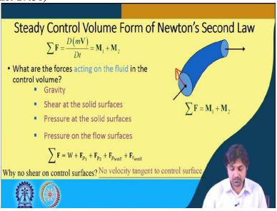
So, now, steady control volume form of Newton's second law, so, this f the net force is the sum of M 1 and M 2 as we already told you in the last slide. So, sigma x where D mV Dt is equal to M 1 + M 2. Now, the question is, what are the forces acting on fluid in the control volume. So, one is gravity, other is shear at solid surface or pressure at solid surface, pressure on the flow surfaces.
