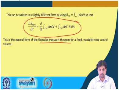
So, starting with the last slide, where we left in the last lecture and the we derived the general form of Reynolds transport theorem here. So, this is the general form and now in the upcoming lecture and slides, what we are going to do is we will apply this Reynolds transport theorem for derivation of different conservation equations.
