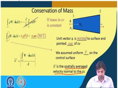
So, now, we are going to see, so, unit vector n cap here is normal to the surface. So, this is the surface 1 which this is normal and on the surface 2 it is in this direction. So, as already indicated by the red arrows, and is pointed out of the control volume in both the cross sections whether it is 1 or 2, the unit vector is normal to the surface and pointed out of the control volume.
