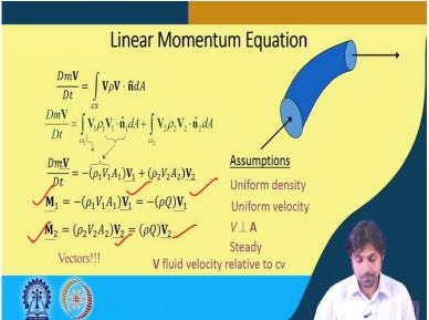
So, now, we similar to the mass we assume cross sections here and we use for the steady state equation, the equation that we have obtained in this slide on the next page. So,
