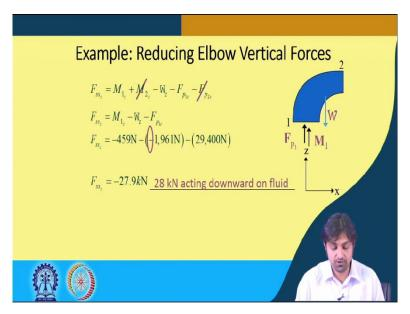
Continuing with our example, we have to find out F ss in z direction or y direction. Basically, we call this one as z. So, M 2 z because this is a horizontal, this is zero and similarly with the pressure force is it is zero. So, F ss z is M 1 - W z - Fp1 z. So, M 1z we found out it was - 459 Newton, weight we already found out and this we just we calculated last time, I mean, in the one slide before. So this minus, minus becomes positive.
