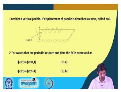
So, consider a vertical paddle if the displacement of the paddle is described as x is a function of s z, t the question is find the kinetic boundary condition. So, this is x is a function of z, t this is the paddle, so, the movement is the next direction of the paddle therefore, we say x = a function of z, t so with this surface equation x - s z, t = 0 are F you can use the similar analysis of the kinematic boundary condition.
