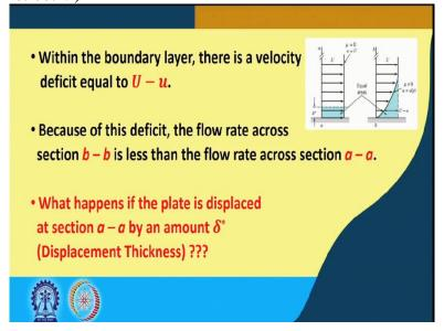
Welcome back to the second lecture of this module, boundary layer analysis. So, last class we finished the lecture by saying, what happens if the plate is displaced at a section a - a by an amount delta dash. So, we displace this plate to here, for example.
