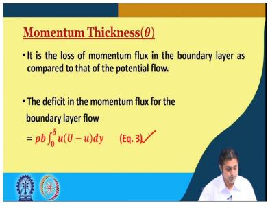
Now, proceeding, what is the momentum thickness theta? So, momentum thickness theta is the loss of momentum flux in the boundary layer, as compared to that of the potential flow. So, there is some loss in the momentum flux. And why that is lost? Because of the presence of the viscosity due to the presence of the plate in a viscous fluid flow. Therefore, this is the loss of the momentum flux.
