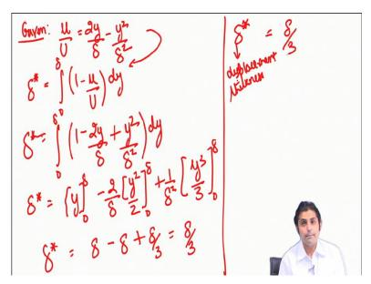
And as always, we start with the thing, that is, given. What is given to us? u / U equal to 2y / delta - y square / delta square. And according to definition of the displacement thickness, that is, delta star, definition is 0 to delta 1- u / U into dy. So, it is quite simple, we use this velocity profile here, we plug it in, and we first write, integral 0 to delta is equal to 1-2y / delta plus, this minus becomes plus, y square / delta square into dy. So, now there are 3 terms to integrate.
