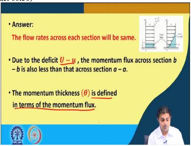
So, to answer that, we see that the flow rate across each section will be the same because the area is the same. But in this section b - b, due to the deficit U - u, the momentum flux across
