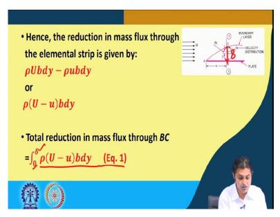
Therefore, the reduction in the mass flux through the elemental strip, compared to the, you know, uniform velocity profile will be the difference of the mass fluxes. This is due to uniform, that is, in the boundary layer, or if we take  $\rho$  outside, b and dy outside, it becomes  $\rho$  into U minus u into bdy.
