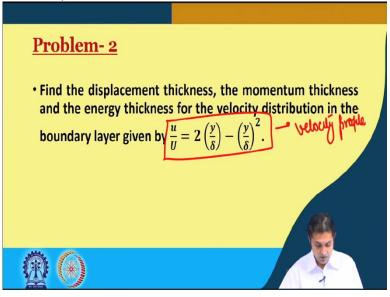
So, we proceed to the next problem. So, our next problem is, find the displacement thickness, the momentum thickness and the energy thickness for the velocity distribution in the boundary layer, that is, given by u / U equal to. So, we have another velocity profile, similar to problem number 1. So, we will solve this problem, as well. So, for doing that we are going to have white screen again.
