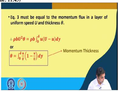
Now, the equation number 3 must be equal to the momentum flux in the layer of uniform speed U and thickness theta. That is how we derive the displacement thickness as well. So, we equate  $\rho$  b U square theta because this is the momentum flux in a layer of uniform speed U and thickness theta, or if we take this down here, as a denominator,  $\rho$  b,  $\rho$  b will get cancelled, this will become
