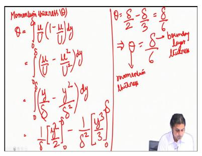
Momentum thickness theta, so, theta definition is equal to 0 to delta u / U into 1- u / U dy and this is going to be 1 to delta. This is going to be u / U – u square / U square into dy and using the velocity profile, we can write, integral 0 to delta u / U is going to be, y / delta minus y square / delta square into dy or removing the integration sign, 1 / delta would come out and this is going to be, y square / z.
