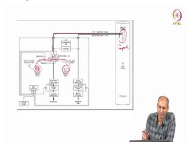
Basically what it what it looks like is this there is a roll of filter paper, the filter paper rolling here, there is a sample inlet that goes in through here and deposits on the filter.
