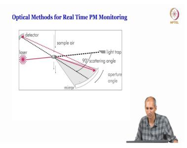
There are other methods of doing real time analysis. I am going to ask a question at the end of this discussion and you have to be prepared for that. There are optical methods in which there is a laser and it is based on scattering principle there is a particle light hits it, it scatters and is based on the scattering law, the amount of scattering and angular scattering depends on the size of the particle. So, different detectors are kept here.
