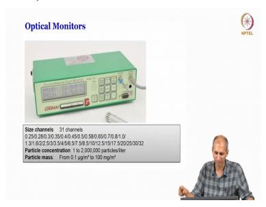
The real time monitor, this will give you very good data because it is measuring it as it is going through, particles are going in and scattering is happening continuously lasers hitting it and you are getting numbers you will get numbers like this and there is a filter at the end of the system which will collect some amount.
