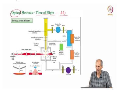
This is a next level of optical instrument. So, this is based on scattering this one there is another instrument which is based on what is called time of flight. This is called as an aerodynamic particle sizer. And as the name suggests this exactly does what the aerodynamic diameter definition is it takes the particle and it finds out what is the momentum of the particle, how fast it is moving a certain size.
