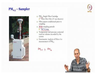
So, this is the other kind of in samplers that that is used, this in this case impactor is here. So, this is the air intake and the impactor is somewhere here, impactor is in this, there is a pump inside. So, this is a PM 2.5 sampler where you can see that because of the design of the impactor the sampling is 24 hours and the flow rate is 16.7 L/min and these are related because the impactor works at a certain flow rate you have to sample for longer that is one. Second is you are also
