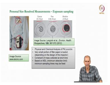
You can also have sizes of cascade impactor this is commercial equipment you can see this here is a small size as cascade impactor. People put this and work for 8 hours they will work and there is a pump here you can see there is a pump and filters in each stage will look like this and you
