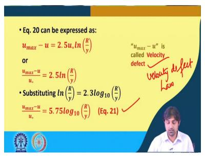
u max, so, what we do is, we bring u on the other side. So, we bring u on this side and we take this whole side component this side, then what the result is, u max minus u because u max will always be larger than u is equal to 2.5 u \*  $\ln R$  / y. y will always be less than R or we bring u frictional velocity down, then we get u max, you bring it down here by dividing then you get u max minus u / u \* equals to  $2.5 \ln R$  / y. And, so, this is  $\ln R$
