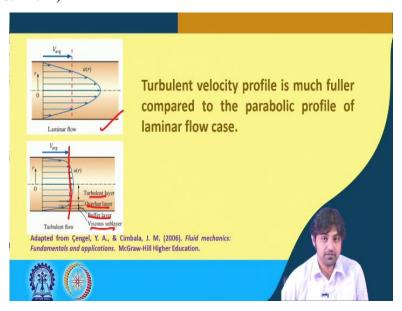
So, now, the turbulent velocity profile is much fuller compared to the parabolic profile of laminar flow case. Actually this is the flow, this is the true picture, this is a laminar flow that we have seen before. But below is, this is the V average and the velocity fluctuates or deviates from these depending upon the flow condition. So, this is the V average line. There are several other
