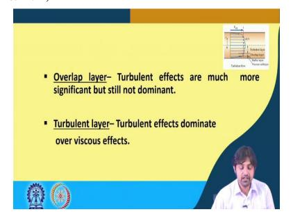
In the overlap layer, the turbulent effects are much more significant but still not dominant, in the overlap layer. In the turbulent layer, the turbulent effects dominate over these viscous effects.
