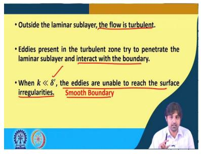
So, outside the laminar sublayer the flow is turbulent, that is, what we have talked about. Eddies present in the turbulent zone try to penetrate the laminar sublayer and interact with the boundary. But when the surface irregularities are much smaller than delta dash, the height of the viscous sublayer, the eddies are unable to reach the surface irregularities when the roughness height is much less. Therefore, we define that boundary as smooth boundary.
