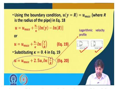
Then using the boundary conditions, what are the boundary conditions? So, u at y is equal to R, where R is the radius of the pipe. We will get, u is equal to u max. That is what we have seen at the center line of the pipe the velocity is going to be the maximum. So, if we use this boundary condition u at y is equal to R is u max, we can get u is equal to, you know, we put u max here, y will be R and therefore, we can obtain C.
