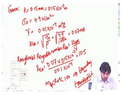
So, we have to write the things that we it has been given to us. k is given as, 0.15 millimeter, it is always a good habit to write it into SI unit into 10 to the power - 3 meter, tau not is actually
