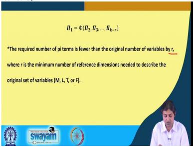
So, Pi 1, this is the first Pi term, so, the final equation is going to be Pi 1 is a function of Pi 2, Pi 3, Pi because this is also dimensionless. Same here, all these things are dimensionless. So, dimensional homogeneity is going to be maintained. So, the required number of Pi terms, it is fewer or lesser than the original number of variables by r. So, k - r, so, the number of dimensionless group would be equal to k - r.
