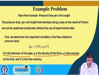
So, let us take an example problem. It is a very, very famous problem, which is an example of the pipe flow. And what we have to determine? We have to determine, pressure drop per unit length. So, we will explore, in principle, how these things can be done using experiments, for example. So, the pressure drop per unit length of the pipe that develops along it, is a result of friction. And this phenomenon cannot be explained analytically without the use of experimental data.
