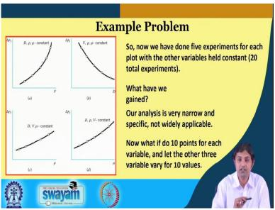
So, this, the hand side is the plot. I am going to explain you what those plot are. So, if you look here, the graph a, what it shows is, that we have varied the flow velocity, we have kept diameter  $\rho$  and  $\mu$  as constant and start measuring the pressure drop per unit length using our apparatus. What we find out is, the pressure drop per unit length is increasing as the velocity is increase. This is a sort of a curve that we are getting.
