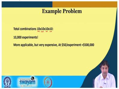
So, total combination because there are 4 variables so, what is going to be our number of experiments? 10 into 10 into 10 into 10. So, there will be 10,000 experiments that we have to conduct and, you know, conducting 10,000 experiments to make it more widely applicable is not a very good idea. I mean, this is definitely possible, but normally it is not preferred. And one of the other, you know, experiments are expensive, very expensive.
