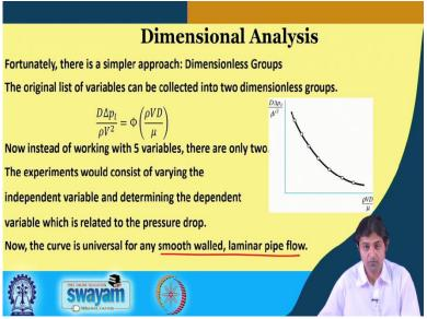
Fortunately, to avoid this, to have, to do, to be able to do less number of experiments, there is a  $\mu$ ch,  $\mu$ ch simpler approach called dimensionless groups or the dimensional analysis. So, this makes our life easy and is therefore the topic for this week's module. So, the original list of variables can, I mean, what happens in dimensional analysis or you know dimensionless groups. The original list of variables can be collected in 2 dimensionless groups.
